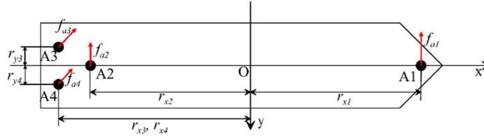
**Fig. 3** Actuators configuration for the reference OSV.
