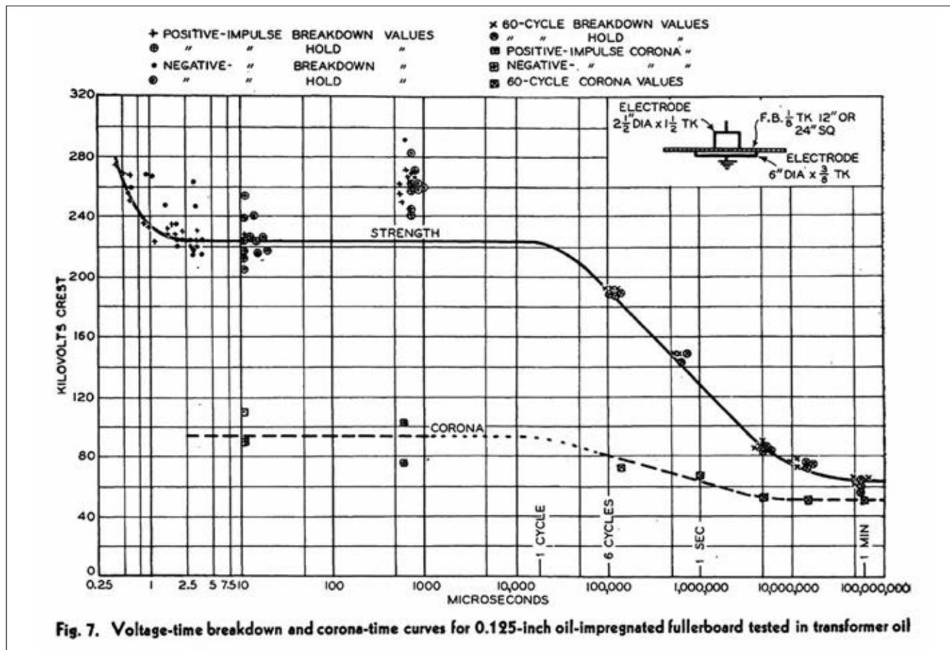
Figure 15. Voltage-time breakdown and corona-time curves for 0.125-inch oil-impregnated fullerboard tested in transformer oil according to [9] = Fig. 7 Bellaschi & Teague [9]
