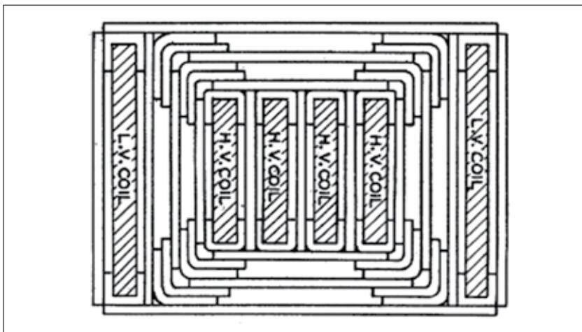
Figure 8. View of a shell-type transformer insulation in iron opening model [8] = Fig. 1 Vogel-1933 [8] High-voltage and low-voltage coils are shaded.
