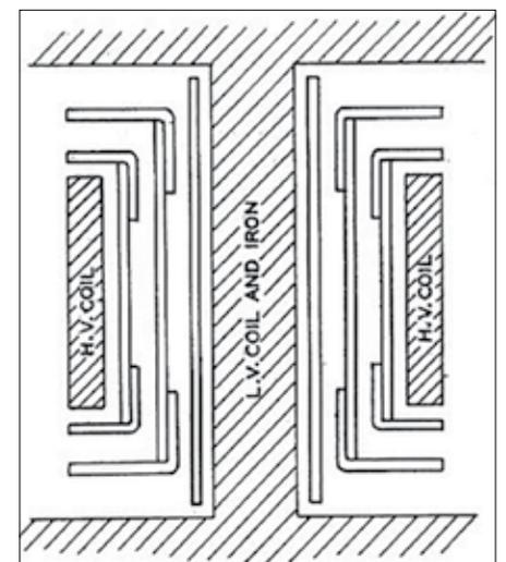
Figure 9. View of core type transformer insulation model [8] = Fig. 2 Vogel-1933 [8] The low-voltage coil and iron are represented as one piece
