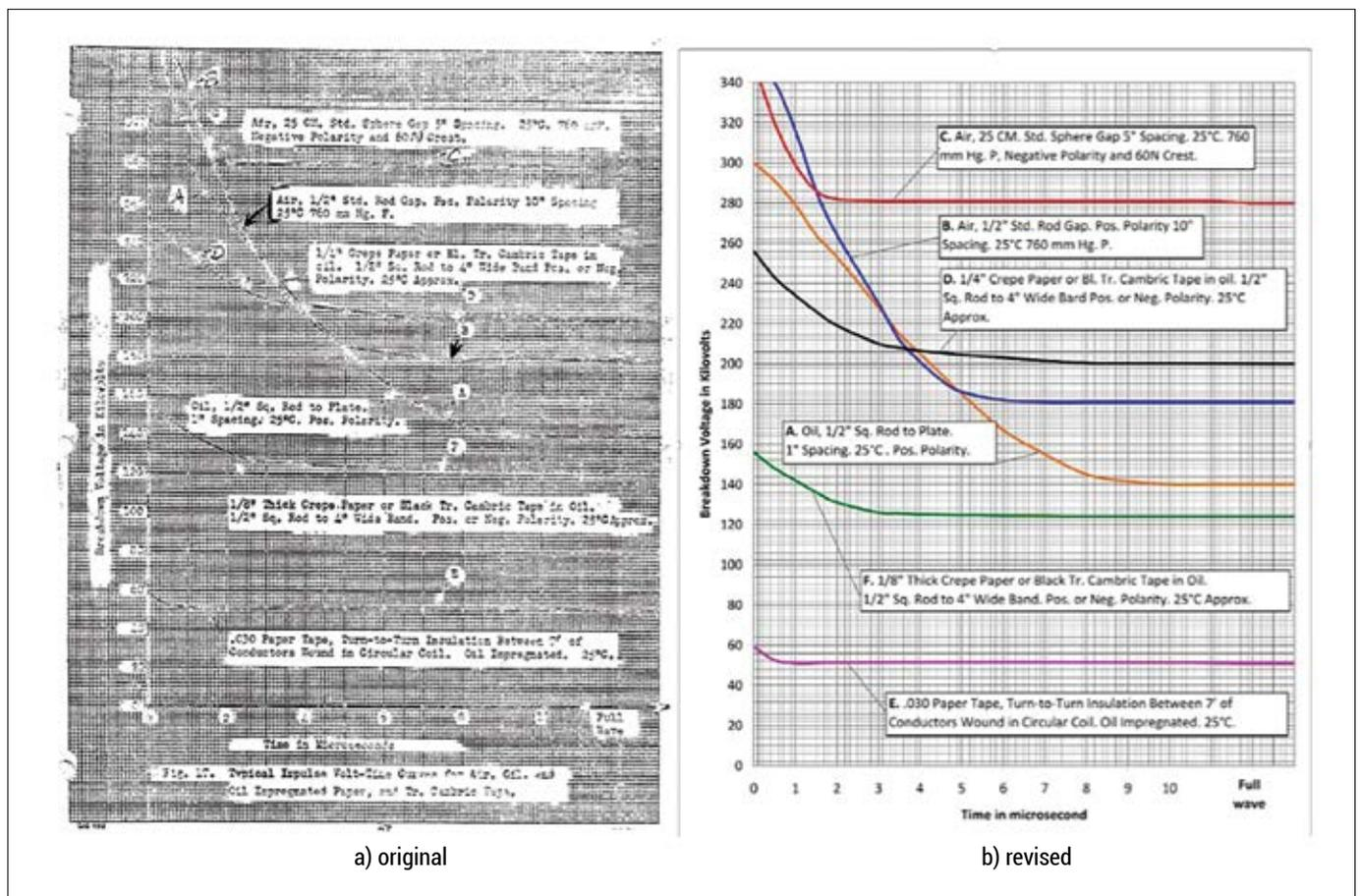
Figure 16. Typical Impulse Volt-Time Curve for Air, Oil and Oil Impregnated Paper, and Tr. Cambric Tape [10] = Fig.17 of Lectures [10]
