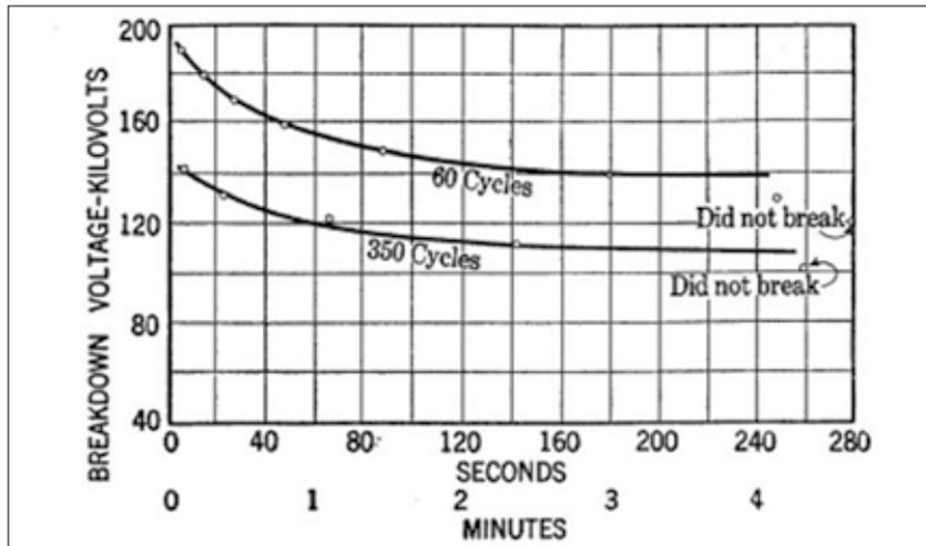
Figure 7. Time-Voltage Curve at 60 and 350 Cycles according to Vogel-1924 [7]. = Fig.25 Vogel-1924 [7] 3 sheets 1/8 in. oil-impregnated fullerboard with alternative 1/8-in. oil ducts at 25°C
