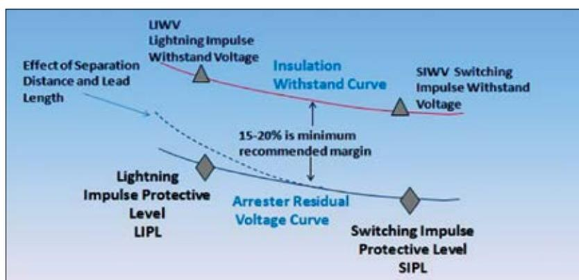
Figure 1. Explanation of margin in the coordination of insulation of modern HV power transformers
