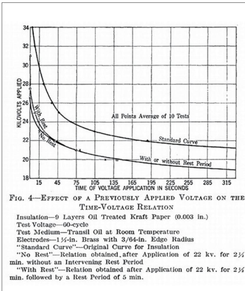
Figure 4. The time-voltage relation of 9 layers of oil-treated kraft paper 0.003 in. acc. to Clark [5]. = Fig. 4 Clark [5]
