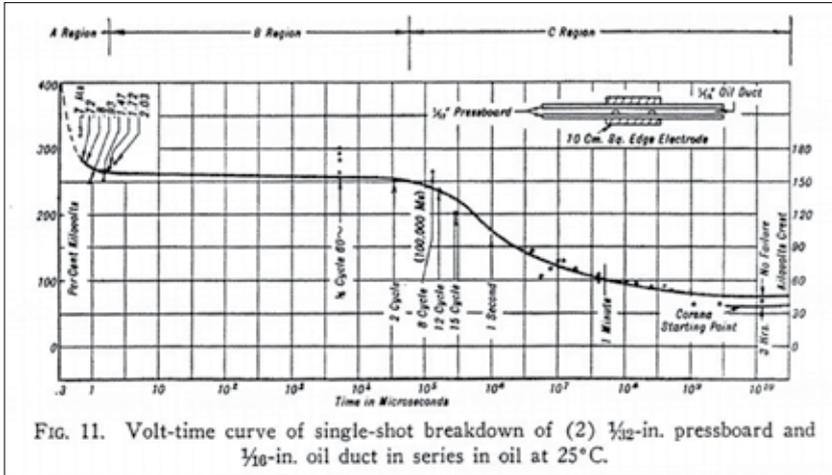
Figure 6. Volt-time curve of single-shot breakdown of (2) 1/32-in. pressboard and 1/16-in. oil duct in series in oil at 25°C = Fig. 11 p. 421 Blume-1951 [6]
