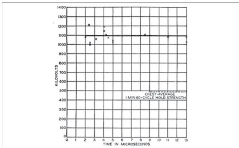
Figure 12. Surge voltage strength of interleaved barrier for both positive (X) and negative (O) waves according to Vogel-1933 [8] = Fig.9 p. 414 Vogel-1933 [8]
