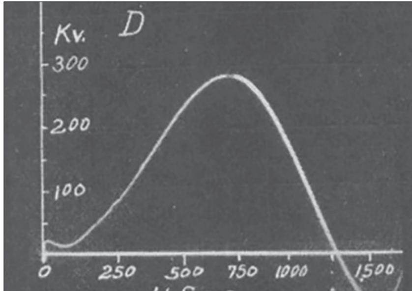
Figure 13. Switching impulse used by Bellaschi & Teague [9] = from Fig. 8 Bellaschi & Teague [9]
