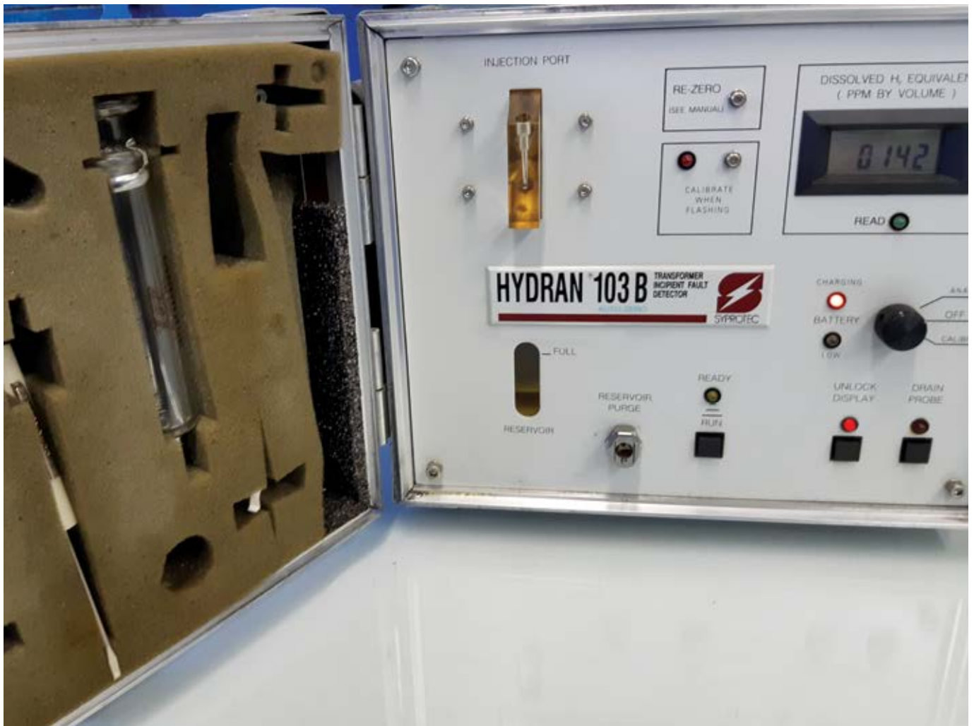
Figure 2. A portable, efficient, and reliable DGA device built with an electrochemical cell. Manufactured by Syprotec
