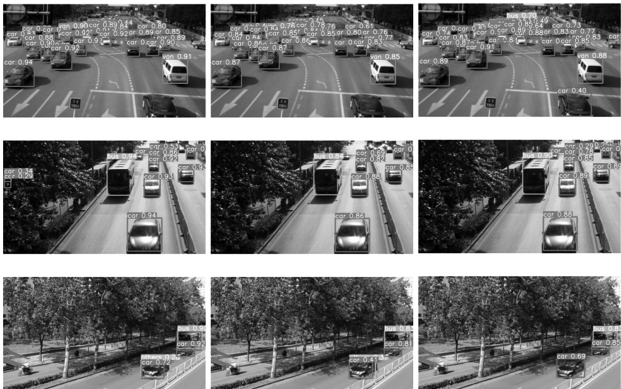
Figure 7. Detection effects of YOLO5s-CIoU (left), YOLO5s-AIoU (middle), and YOLO5s-SAG-AIoU (right).
