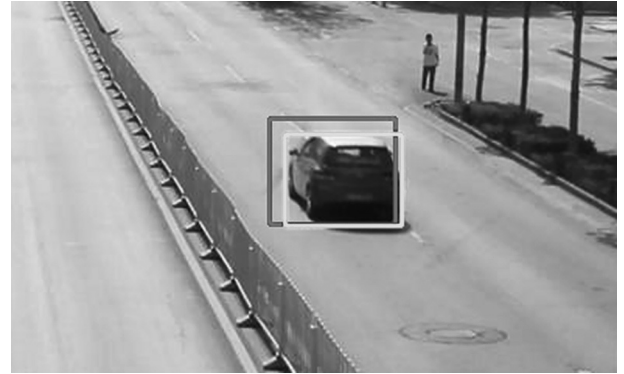
Figure 3. Difference between target box and detection box trained by CIoU.
