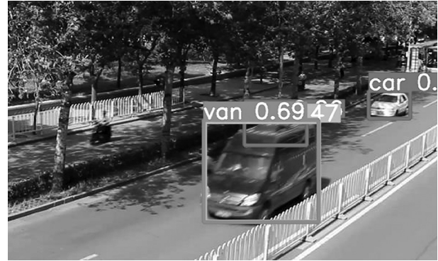
Figure 4. Instances of single targets marked by multi-category detection boxes.
