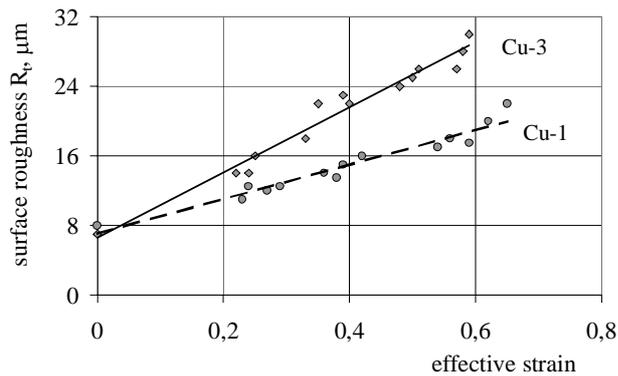
Fig. 1 The value of surface roughness parameter  $R_r$  as a function of effective strain, after incremental straining of copper sheets in the tensile tension test and biaxial stretching
