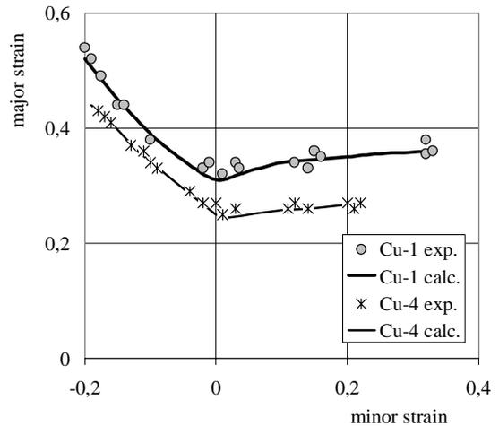
Fig. 4 Comparison between experimentally determined limit strains and calculated FLC of fine grained (Cu-1) and coarse grained (Cu-4) copper sheets
