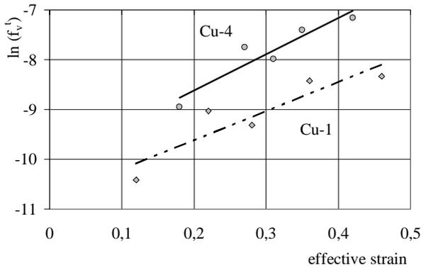
Fig. 2 Volume fraction of material defects as a function of effective strain of copper sheets deformed in uniaxial tension and equibiaxial stretching
