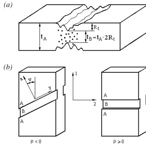
Fig. 3 Schematic representation of the material model: (a) sheet element with geometric imperfections caused by surface roughness and internal defects concentrated in weak band B; (b) orientation of the weak band B according to principal strain
