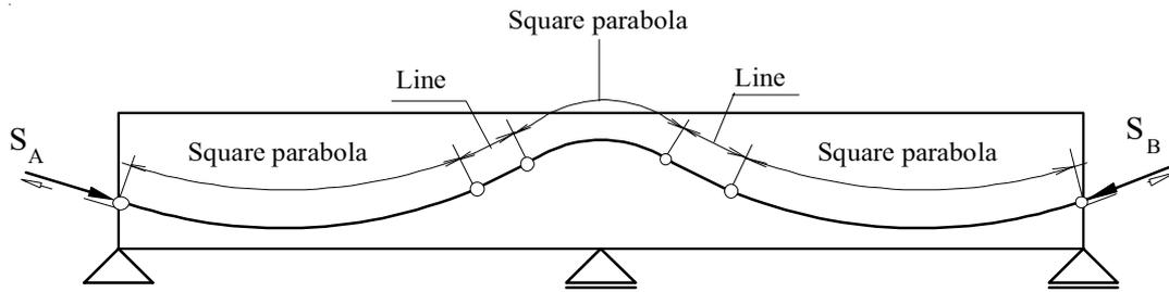
Fig. 1 Possibility of tendon determination for two-dimensional analysis
