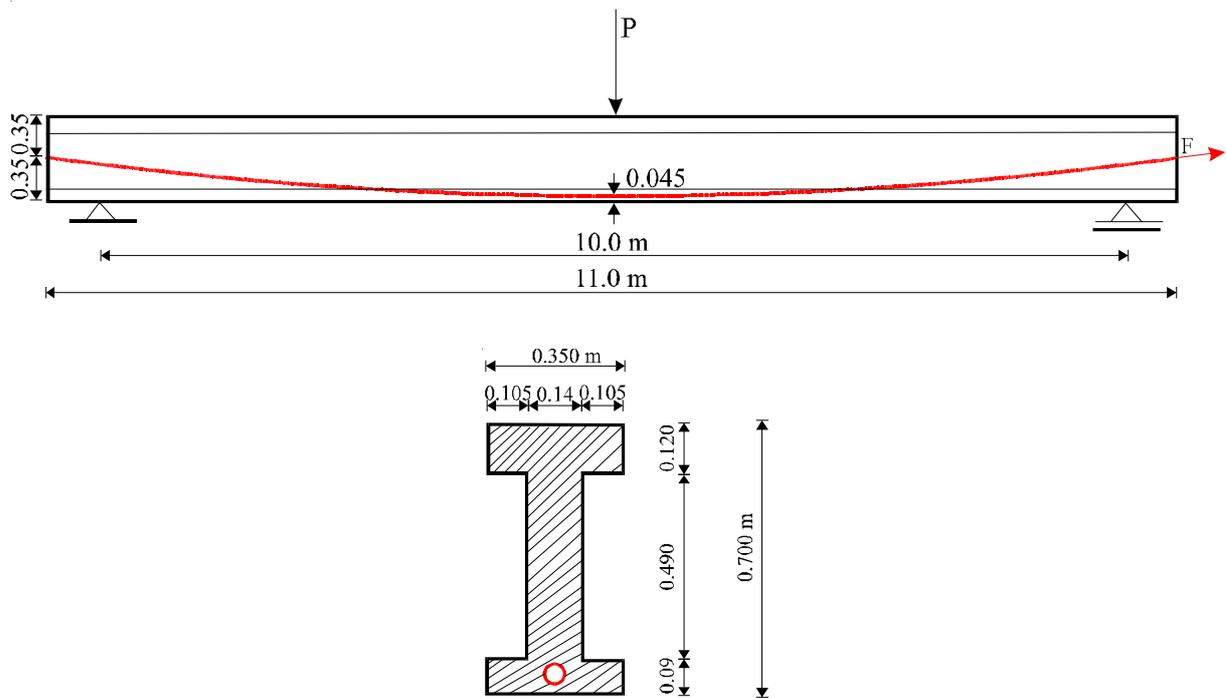
Fig. 8 Geometry of the analysed I-beam
