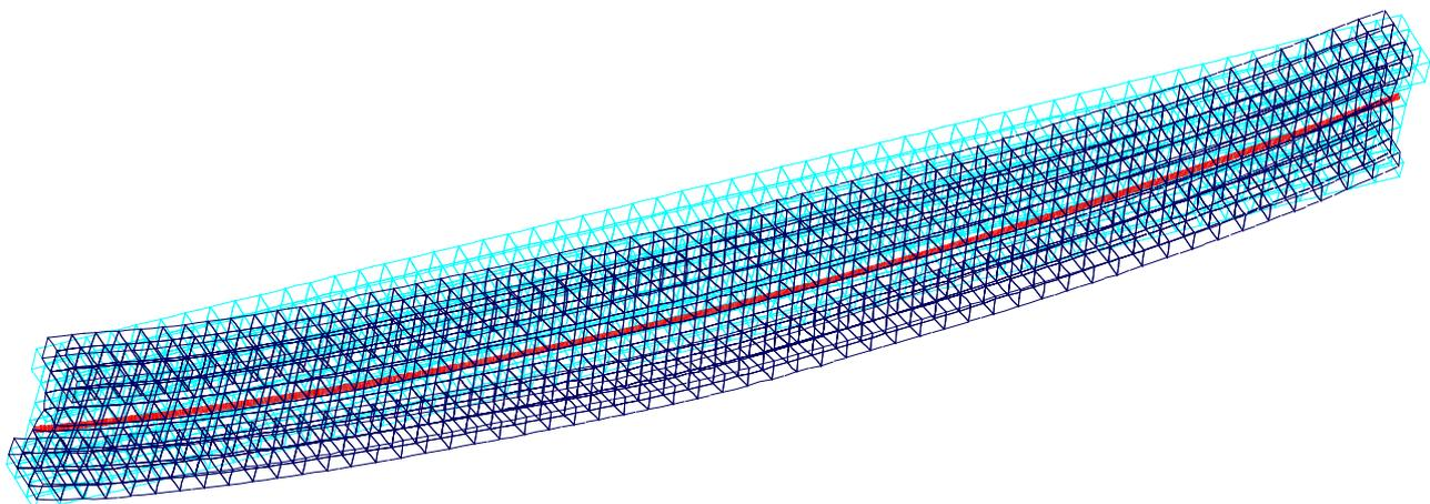
Fig. 10 Deformed configuration of the I-beam under concentrated force acting after prestressing occur
