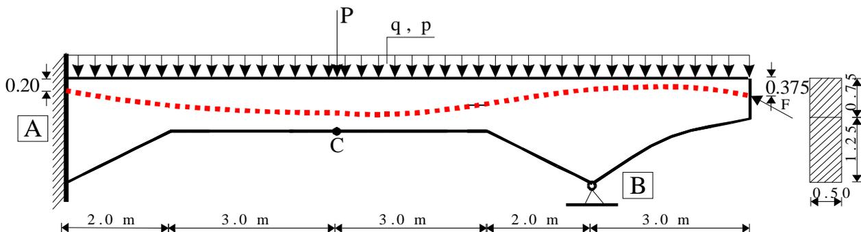
Fig. 6 Geometry of the girder and loadings
