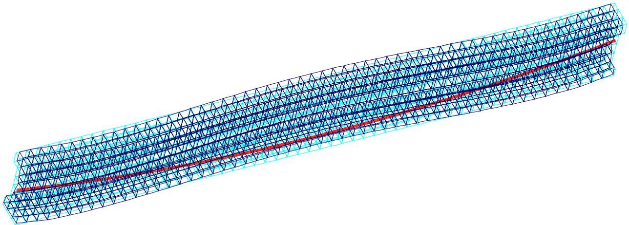
Fig. 9 Deformed configuration of the I-beam under prestressing force
