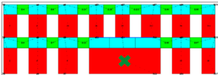
12 Prediction given by Tremuri for the south facade. The green cross indicates that element 25 failed in shear (drawing: Thibaud Maillard, 2023)
