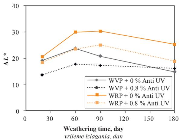
**Figure 6**  $\Delta L^*$  factor variation of WPC made from virgin and recycled polypropylene
