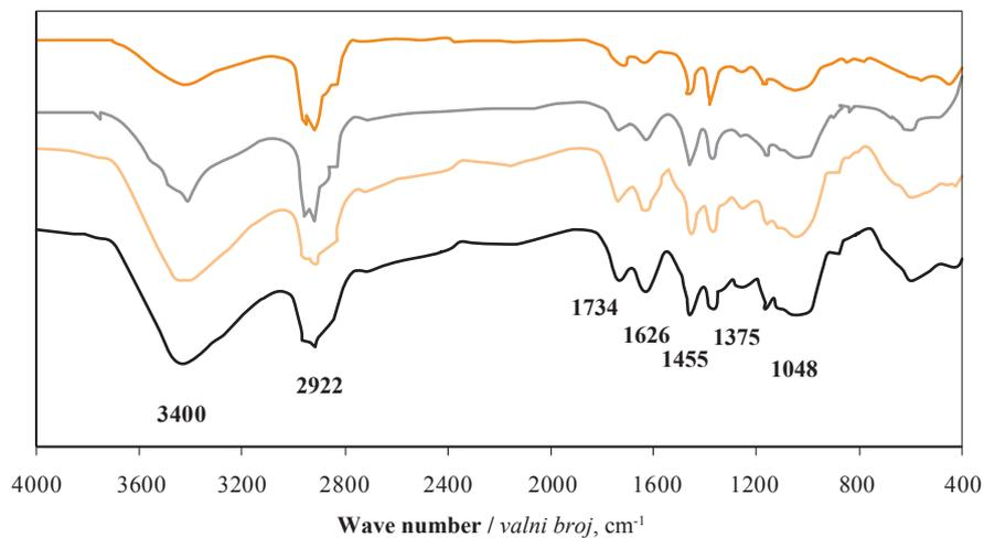
**Figure 9** Effect of natural weathering on FTIR spectrum of WPCs made from recycled PP with 0.8 % UVA: before weathering (a), after 90 days of weathering (b), after 180 days of weathering (c), and after 270 days of weathering (d)
