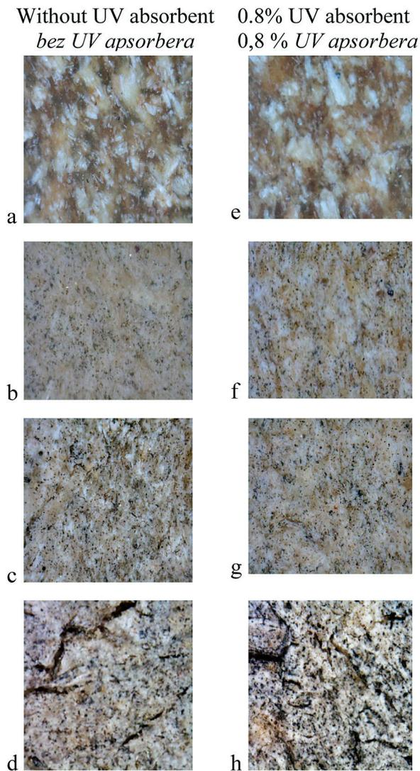
**Figure 1** Microscopic images of WPC surface made from virgin polypropylene before natural weathering (a and e), after 90 days (b and f), after 180 days (c-g), and after 270 days (d and h) of natural weathering
