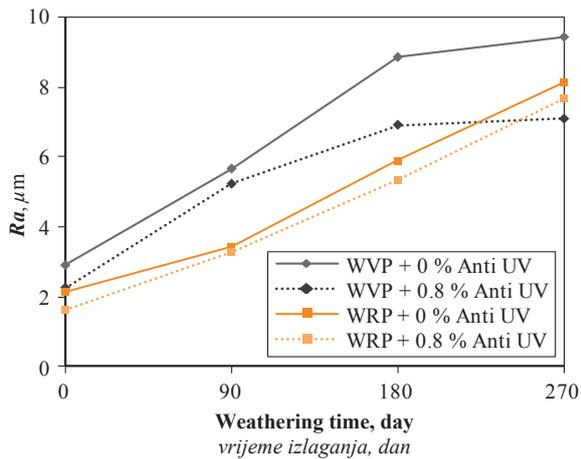
**Figure 3**  $R_a$  variation of WPC surfaces made from virgin and recycled polypropylene
