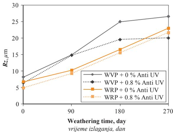
**Figure 4**  $R_z$  variation of WPC surfaces made from virgin and recycled polypropylene
