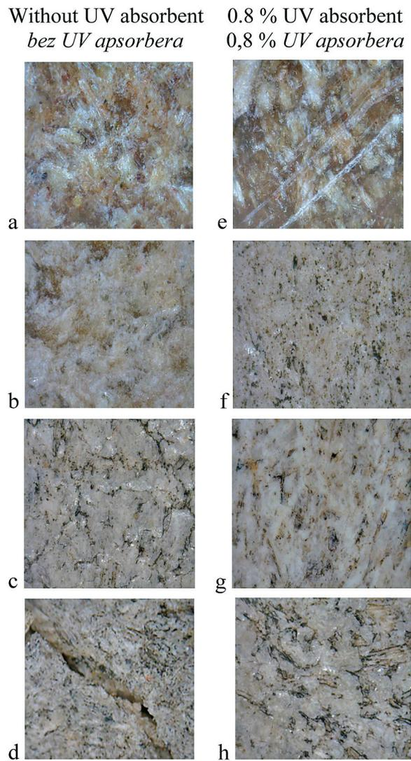
**Figure 2** Microscopic images of WPC surface made from recycled polypropylene before natural weathering (a and e), after 90 days (b and f), after 180 days (c-g), and after 270 days (d and h) of natural weathering
