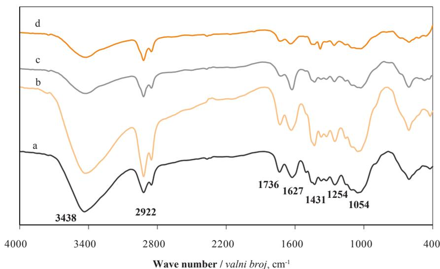
**Figure 8** Effect of natural weathering on FTIR spectrum of WPCs made from virgin PP with 0.8 % UVA: before weathering (a), after 90 days of weathering (b), after 180 days of weathering (c), and after 270 days of weathering (d)
