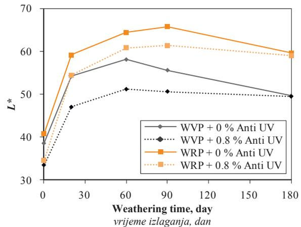
**Figure 5**  $L^*$  factor variation of WPC made from virgin and recycled polypropylene
