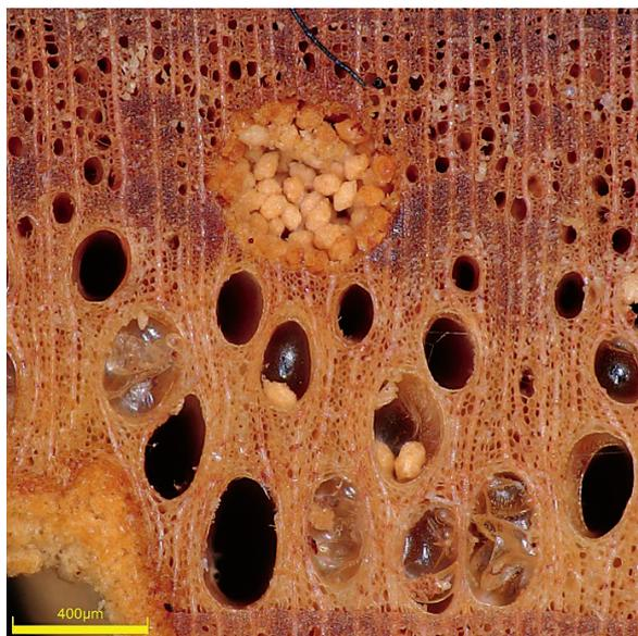
**Figure 9** Insect hole in sweet chestnut wood filled with debris typical for beetles from genus *Anobium*
