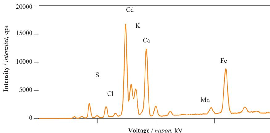
**Figure 11** Representative XRF spectra of wood from mill interior
