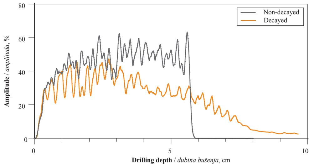
**Figure 8** Resistograph profiles of non-decayed and decayed beam in the analysed mill
