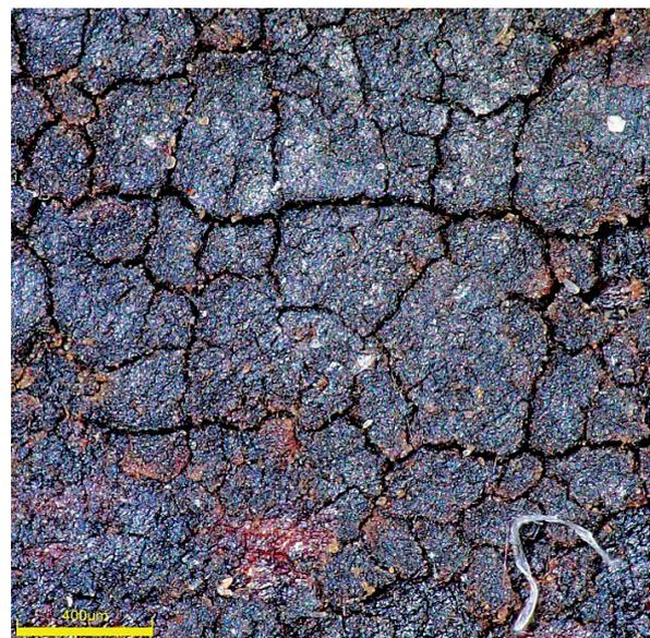
**Figure 10** Deposits on oak beams surface in mill interior
