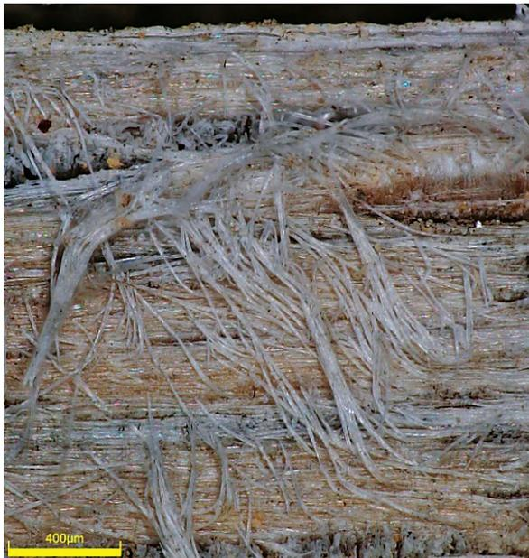
**Figure 6** Presence of loose cellulose fibres on weathered wood surface
