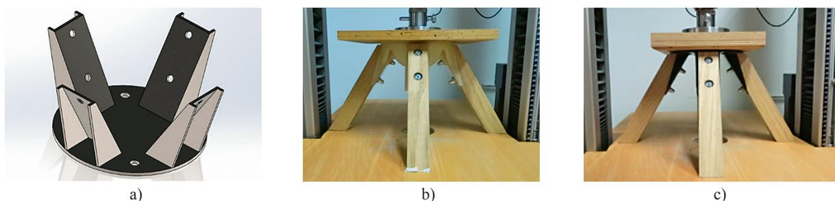
**Figure 2** a) 3D model of connector (SolidWorks), b) connector made of PLA material, c) connector made of metal (Cvetko, 2020)
