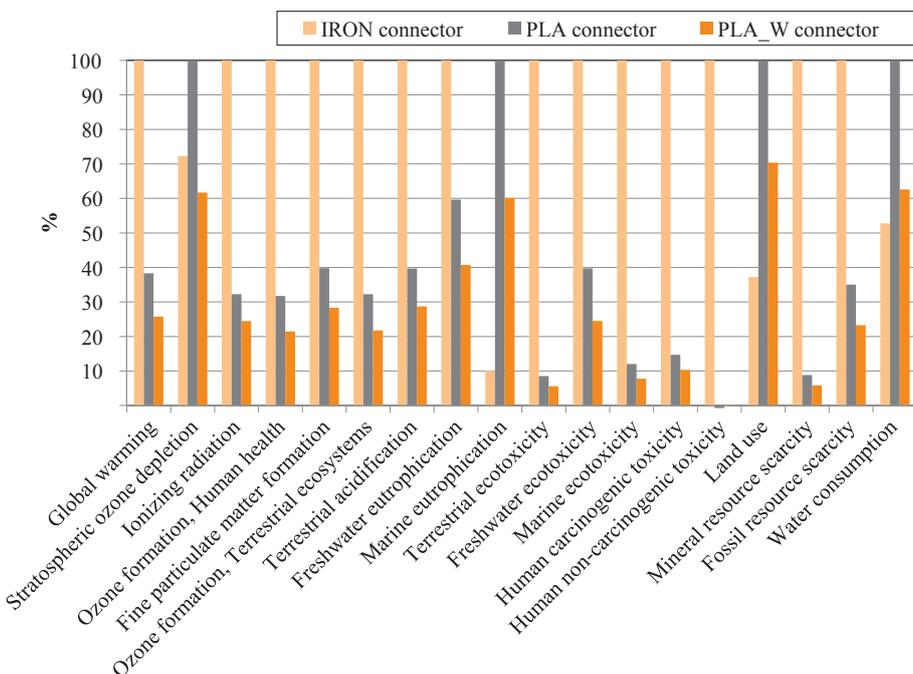
**Figure 5** Impact assessment of 3 versions of chair connectors using ReCiPe 2016 Midpoint (H) method with characterization of results, excluding long-term emissions
