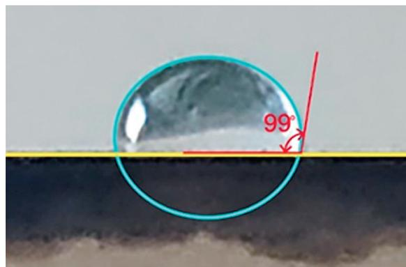
**Figure 2** Behaviour of liquid (distilled water) in contact with bio-based coating surface (static water contact angle  $\theta$  is  $99^\circ$ )
