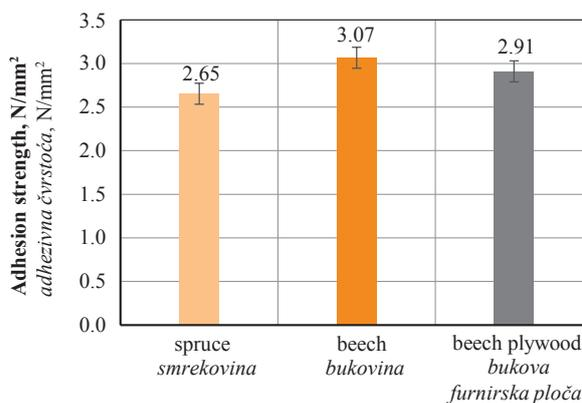
**Figure 5** Adhesion strength of wood samples coated with two-layer bio-based stain
