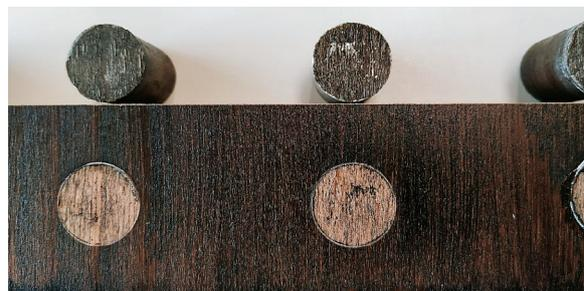
**Figure 4** Typical destruction after axial pull-off test
