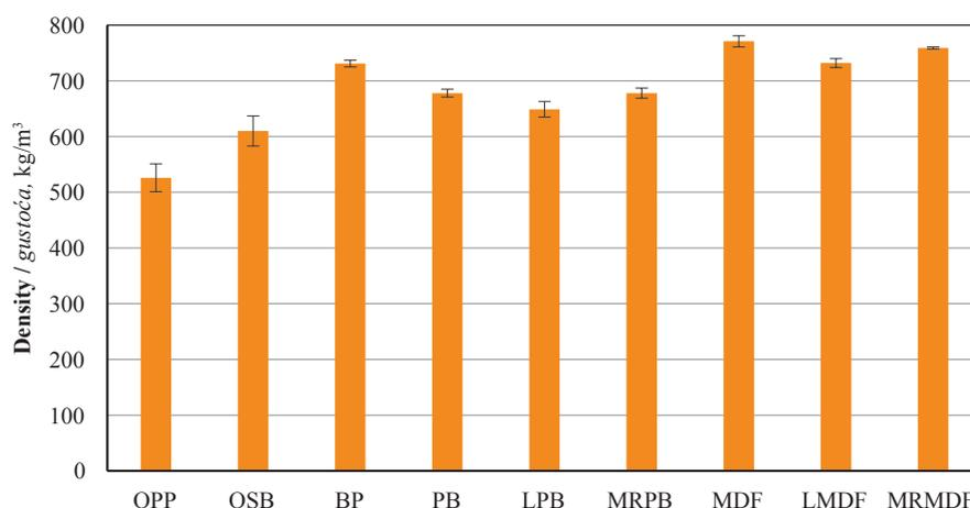
**Figure 1** Density of tested specimens - oak-pine shield parquet (OPP), oriented strand board (OSB), birch plywood (BP), particle board (PB), laminated particle board (LPB), moisture-resistant particle board (MRPB), medium density fibreboard (MDF), laminated medium density fibreboard (LMDF), moisture resistant medium density fibreboard (MRMDF)
