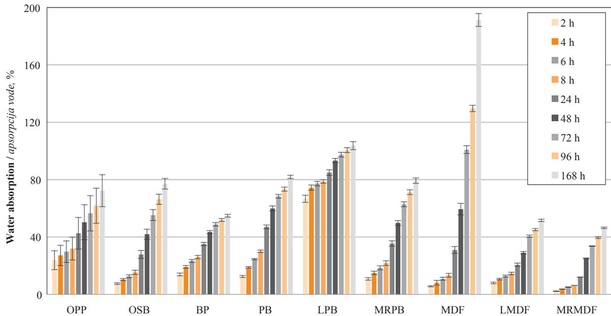
**Figure 2** Water absorption of tested specimens after 2 h to 168 h - oak-pine shield parquet (OPP), oriented strand board (OSB), birch plywood (BP), particle board (PB), laminated particle board (LPB), moisture resistant particle board (MRPB), medium density fibreboard (MDF), laminated medium density fibreboard (LMDF), moisture resistant medium density fibreboard (MRMDF)
