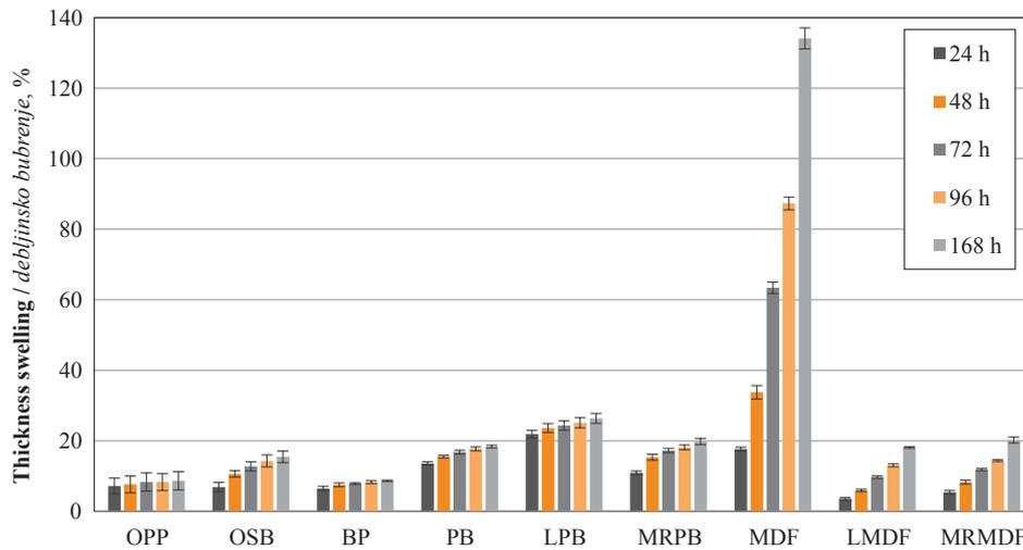
**Figure 3** Thickness swelling after 24 h to 168 h immersion in water of tested specimens - oak-pine shield parquet (OPP), oriented strand board (OSB), birch plywood (BP), particle board (PB), laminated particle board (LPB), moisture resistant particle board (MRPB), medium density fibreboard (MDF), laminated medium density fibreboard (LMDF), moisture resistant medium density fibreboard (MRMDF)
