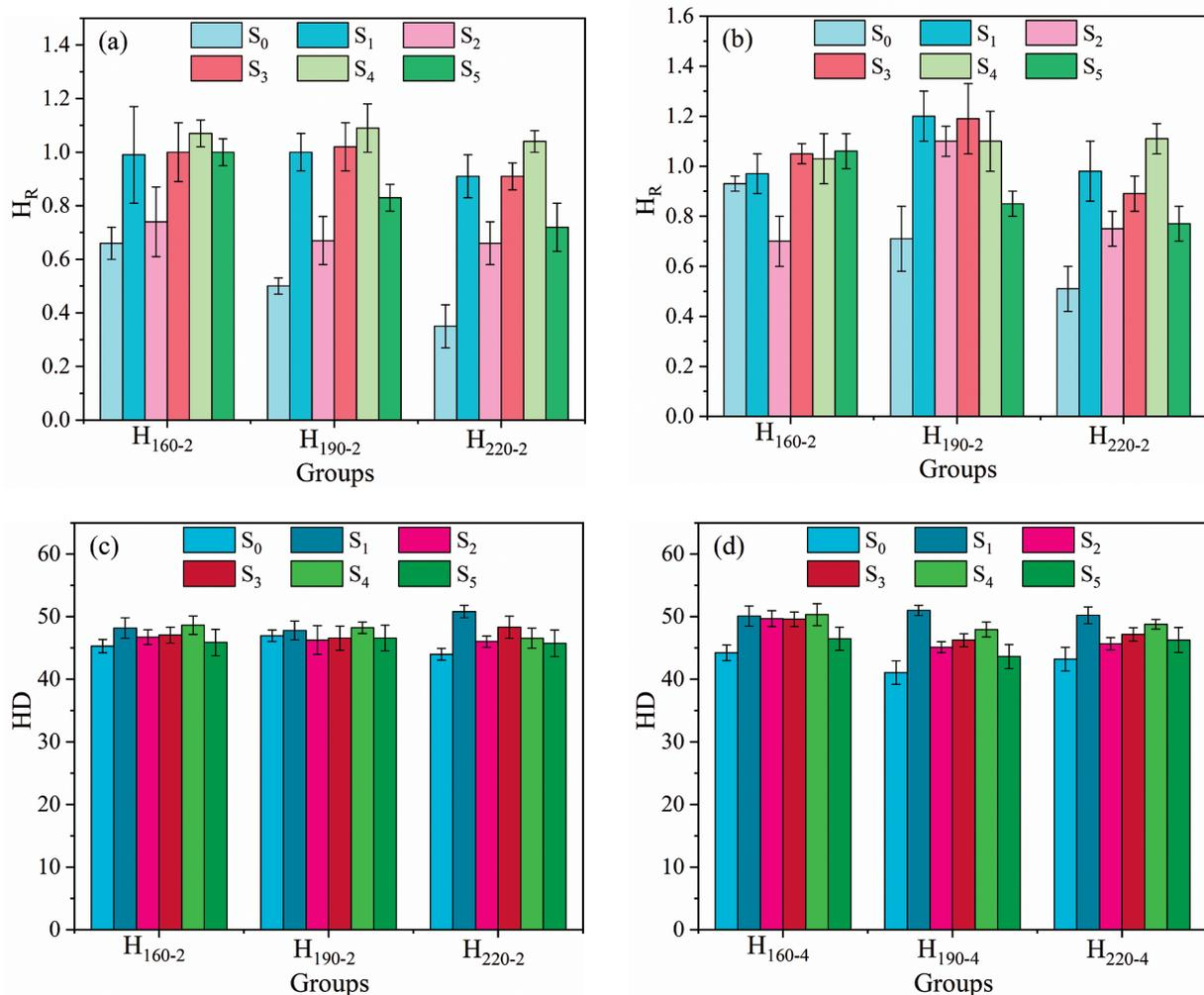
**Figure 3** Surface pressure ball and Shore hardness of test layers in different positions of heat-treated poplar board
