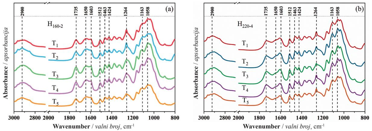
**Figure 4** Infrared spectra of different surface layers of heat-treated poplar wood
