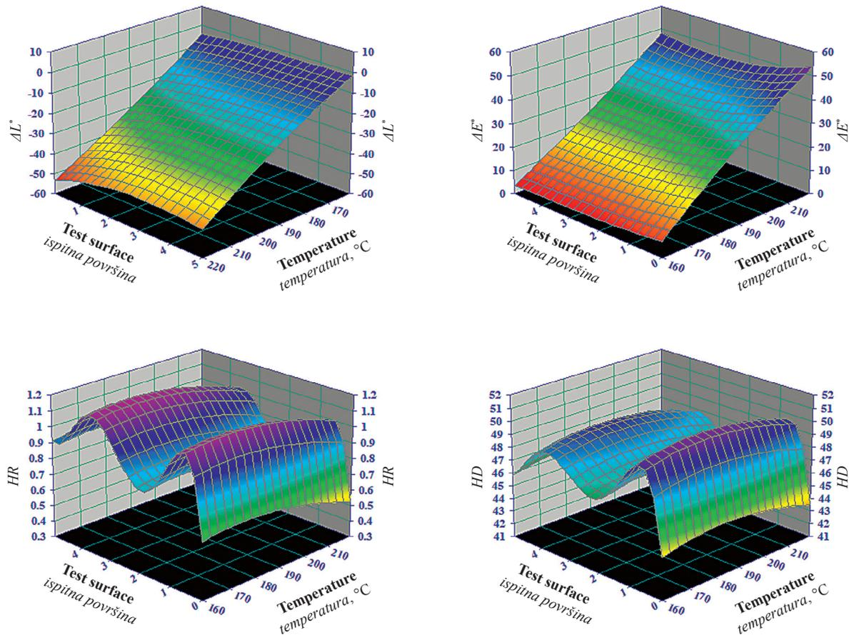
**Figure 5** Fitting surface of  $\Delta L^*$ ,  $\Delta E^*$ ,  $H_R$ ,  $HD$  of heat-treated poplar board
