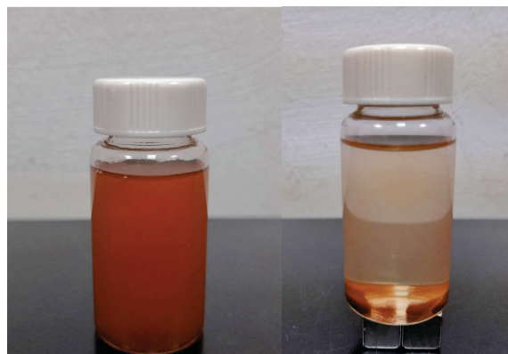
Figure 2. Photographs of magnetic separation of Fe 3 O 4 by an external magnet at the end of the adsorption.
