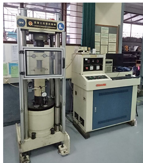
Figure 5: Hungta Machine of 200 kN, ITB Geomechanics and Mining Equipment Laboratory.
