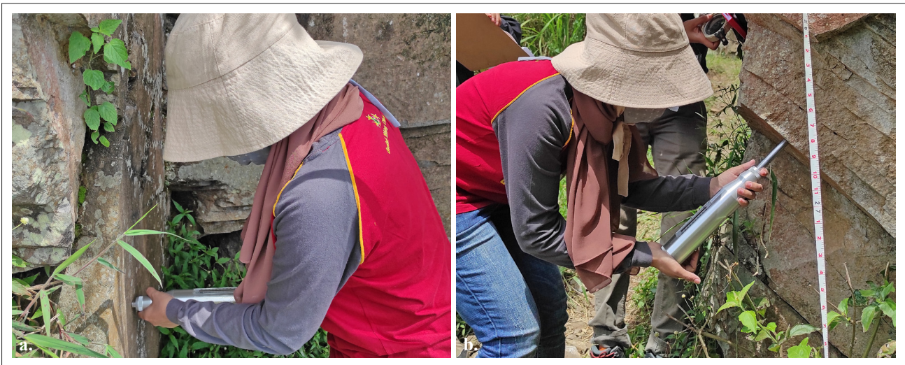
Figure 4: Schmidt hammer type N test.
