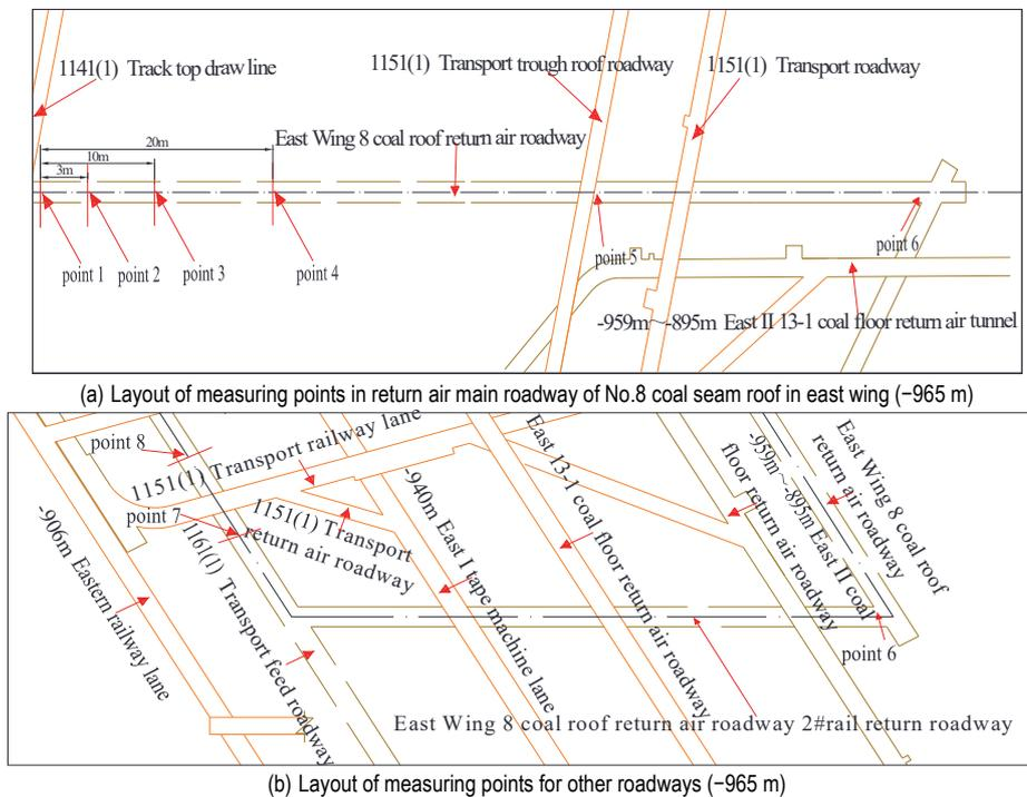
Figure 5 Layout of measuring points of roadway thermal environment
