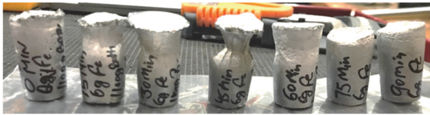
Figure 2 Batch No. 2 Samples - Iron saturated Al-Zn melt (starting bath 0.20% Fe and then Fe concentration raised to 0.40%)
