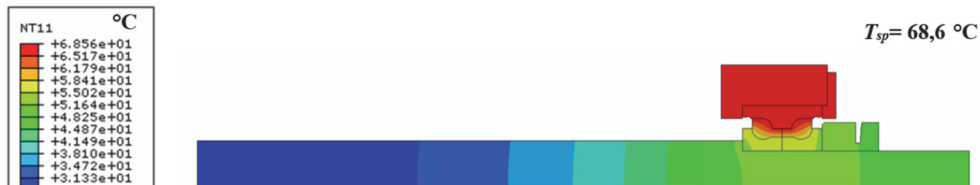
Figure 11 Bearing assembly's temperature field with steel housing
