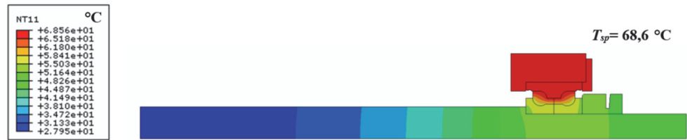
Figure 13 Bearing assembly's temperature field with grey cast housing
