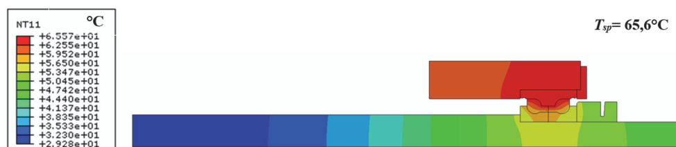
Figure 15 Bearing assembly's temperature field with twice the length of the steel housing compared to previous models
