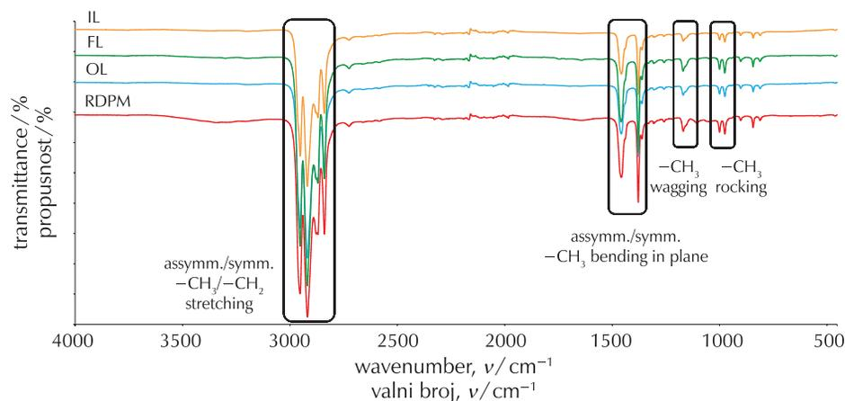
Fig. 3 – Comparison of the FT-IR spectra of IL, FL, OL, and RDPM samples
