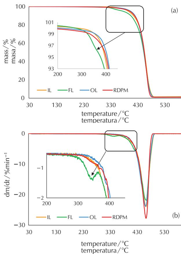
Fig. 6 – Comparison of (a) TG, and (b) DTG curves of the investigated samples
