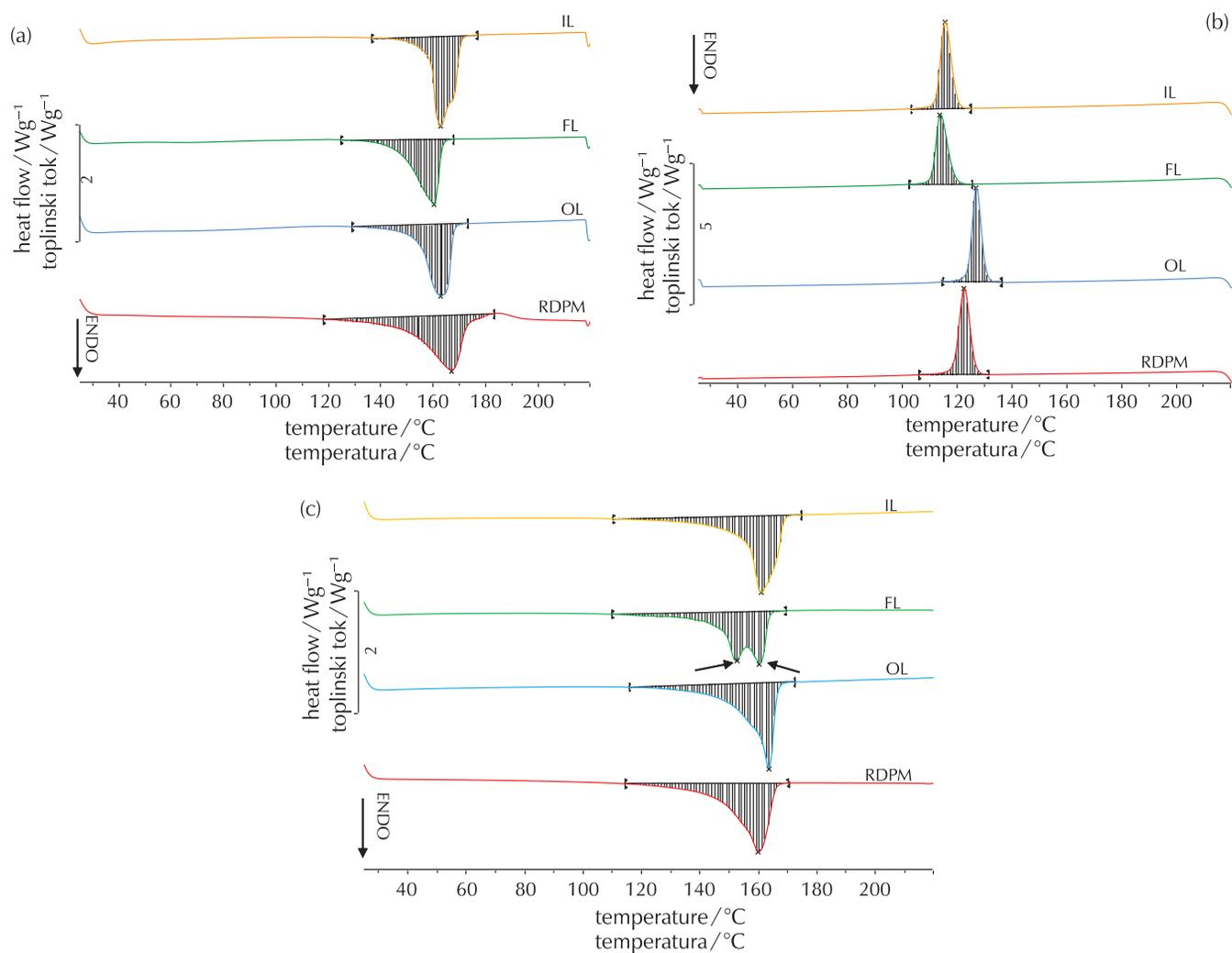
Fig. 4 – Comparison of the normalised DSC curves of the investigated samples: (a) first heating, (b) cooling, and (c) second heating
