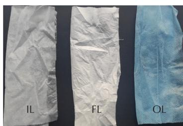
Fig. 2 – Three individual layers separated from the fabric material of the mask
