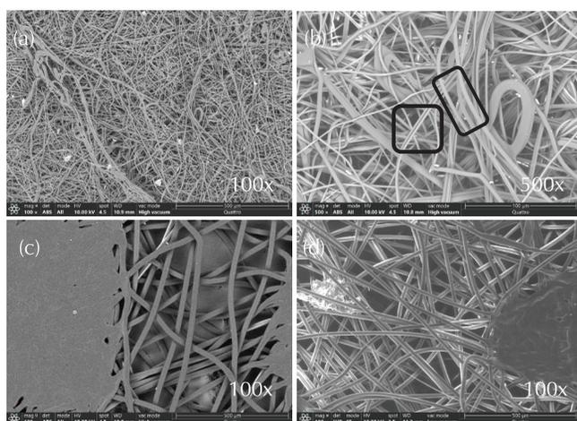
Fig. 5 – SEM micrographs of (a) FL, (b) FL (500× magnification), (c) OL, and (d) IL samples
