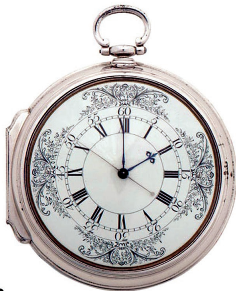
Sl. 3. H4 – Harrisonov usavršeni model kronometra (a) i K1 – Kendallova kopija Harrisonova modela H4 (b) Izvor: http://www.nmm.ac.uk/server/show/conWebDoc.355 , 11. 02. 2008.
