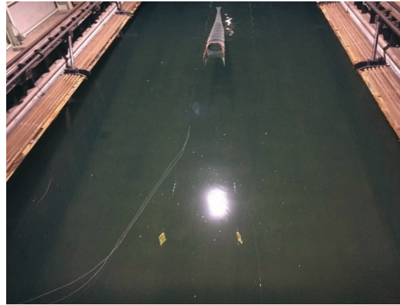
Fig. 5 Experimental test of the trawl model by Su (Source: Su Zhi Peng)
