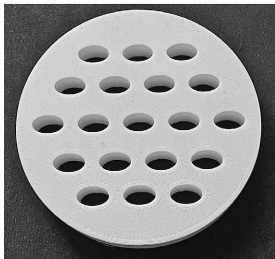
Figure 1 Multi-hole ceramic filter used for testing.
