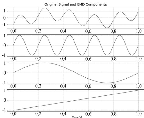
Figure 1 The EMD decomposition diagram
