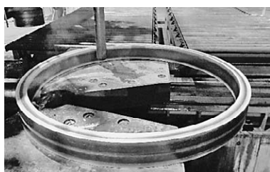
Figure 1 Shaped by rolling a ring of EN AW – 7075
