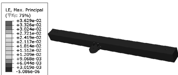
Figure 7 Plastic deformation diagram of the balance beam
