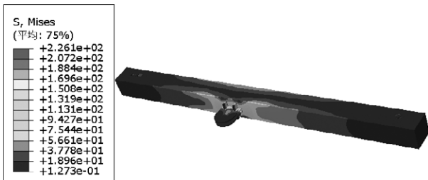
Figure 5 Stress diagram of the balance beam
