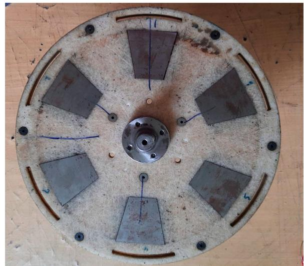
**Figure 19.** Segmented rotor poles embedded in Epoxy Resin Laminate.
