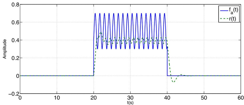
Figure 2. Residual and actuator fault signal.
