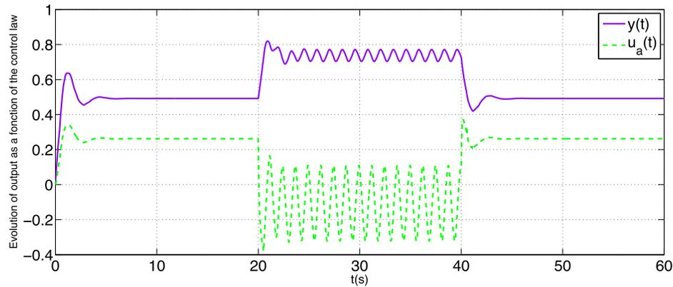
**Figure 8.** Output signal with  $u_a(t)$  control law.
