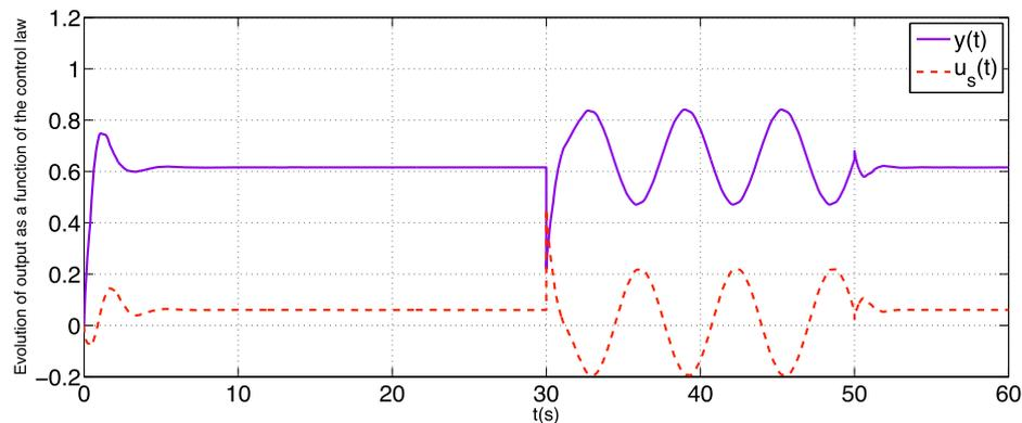
**Figure 9.** Output signal with  $u_s(t)$  control law.
