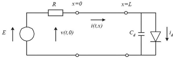
Figure 1. Transmission line circuit.
