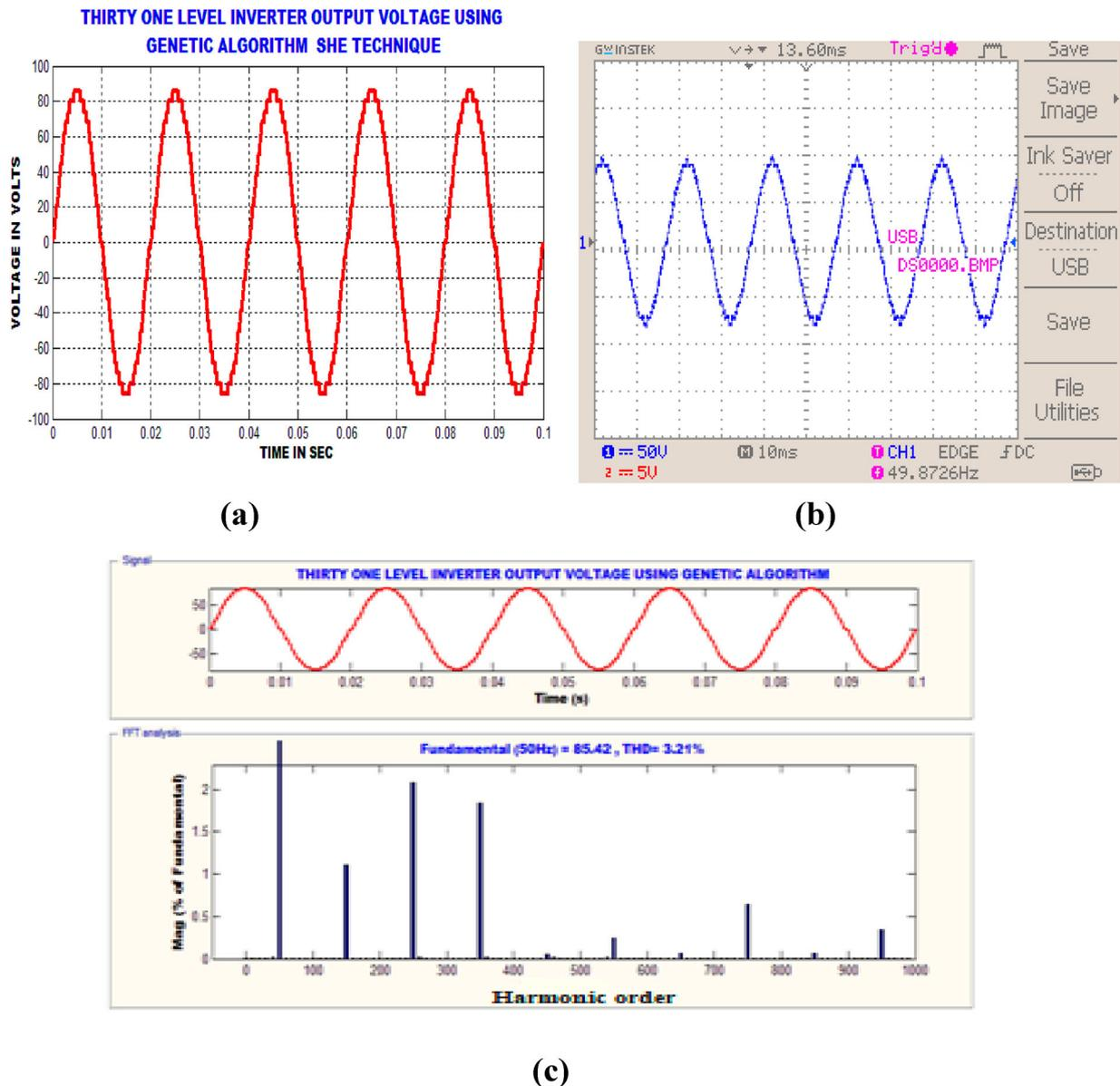
**Figure 14.** (a) Simulation output voltage 31-level inverter using GA technique (b) Hardware output voltage 31-level inverter using GA (c) FFT analyse of 31-level inverter using GA technique.
