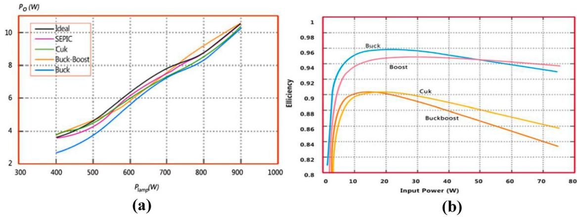
Figure 4. (a) Comparing the tracking capabilities of the different converters. (b) Efficiencies of four DC–DC converter configurations.
