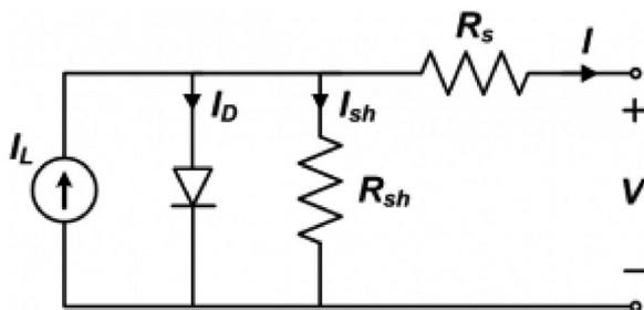
Figure 2. One diode model of the PV system.
