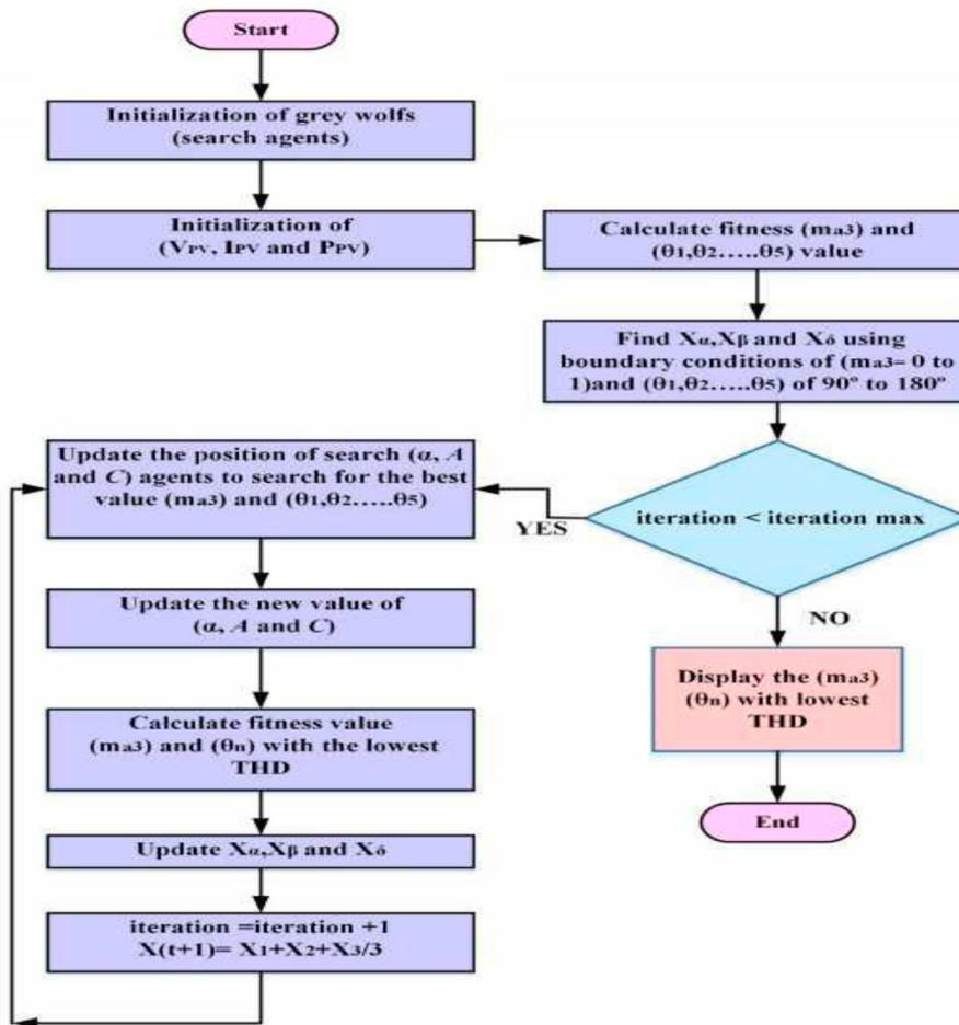
Figure 5. Flow chart for GWO-based optimization algorithm.
