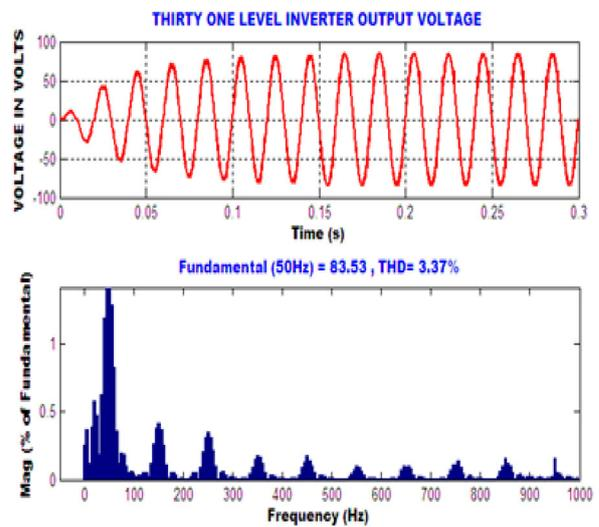
Figure 12. Simulation THD result of 31-level inverter using MCM technique.
