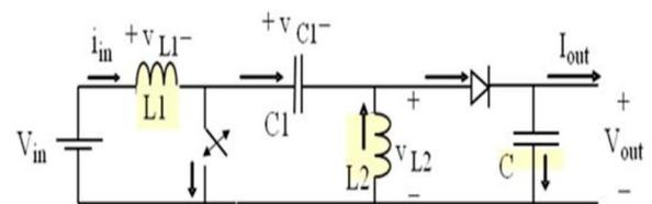
Figure 3. Proposed SEPIC converter circuit diagram.
