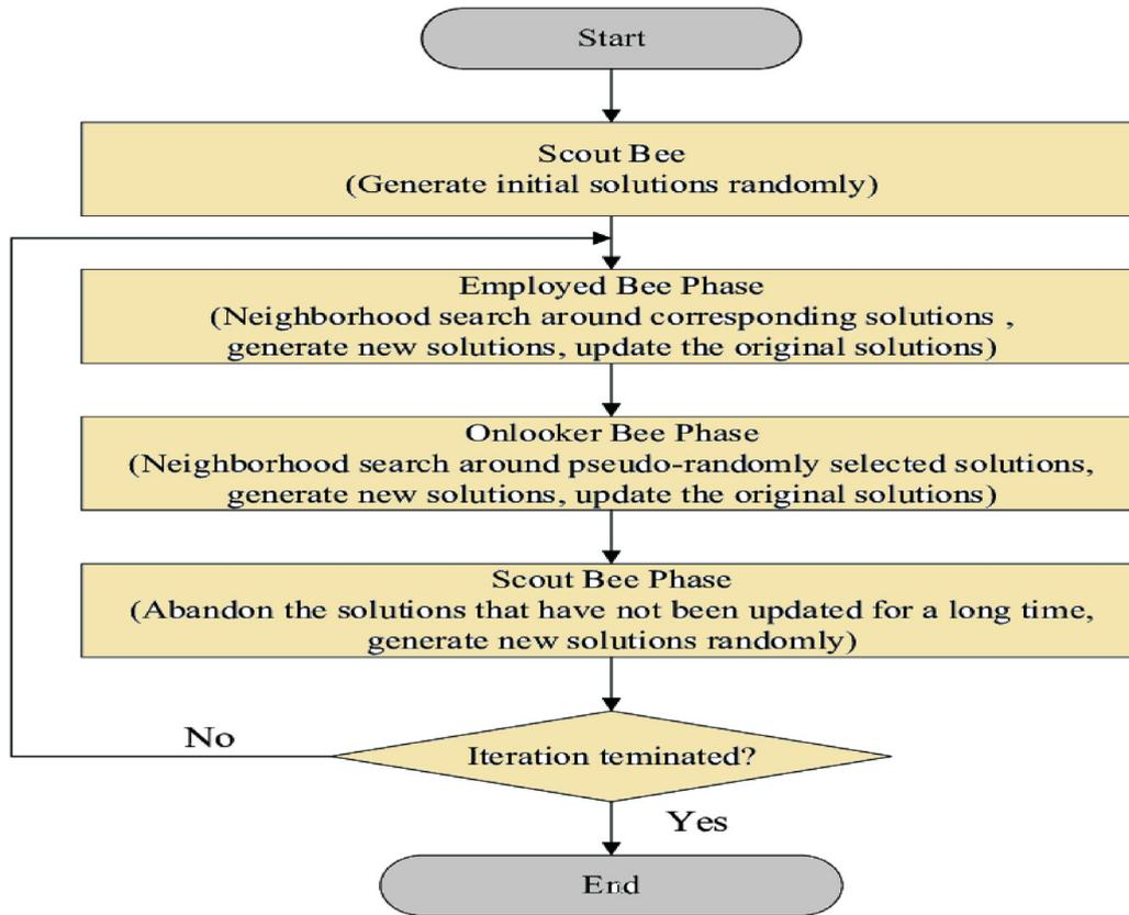
Figure 7. Flow chart for ABC-based optimization algorithm.
