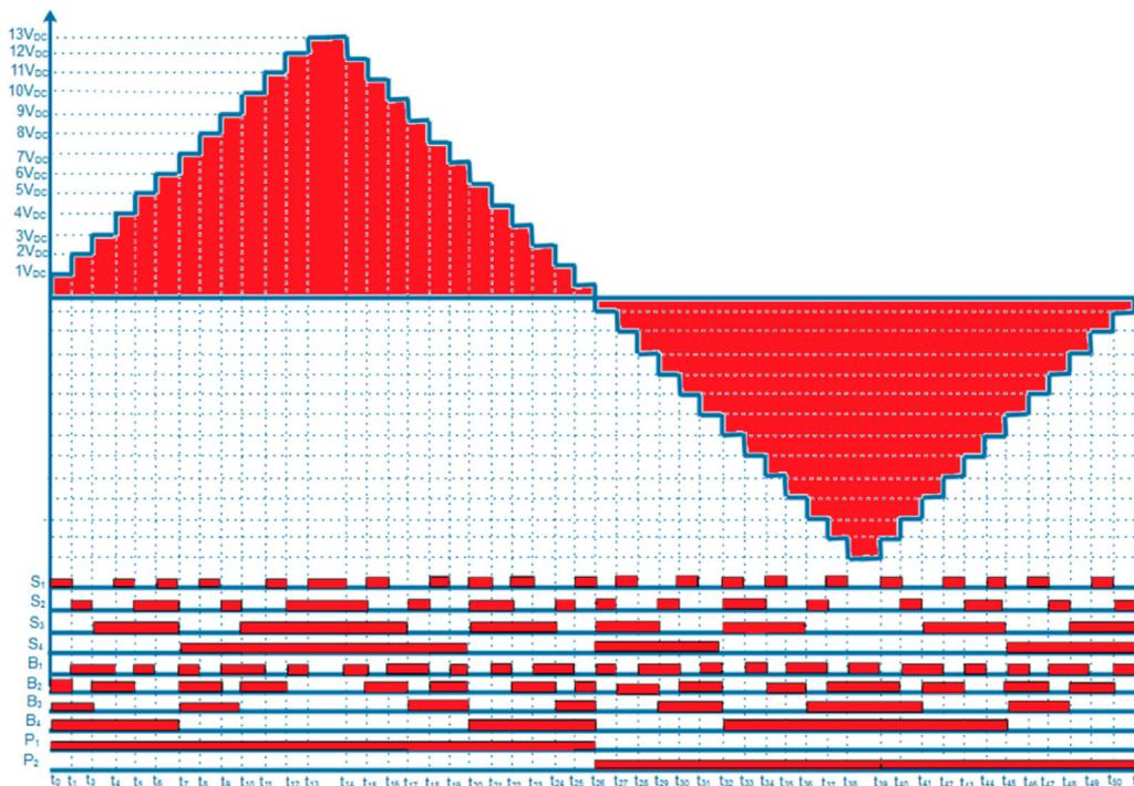
**Figure 6.** Angle generation for 31-level inverter.
