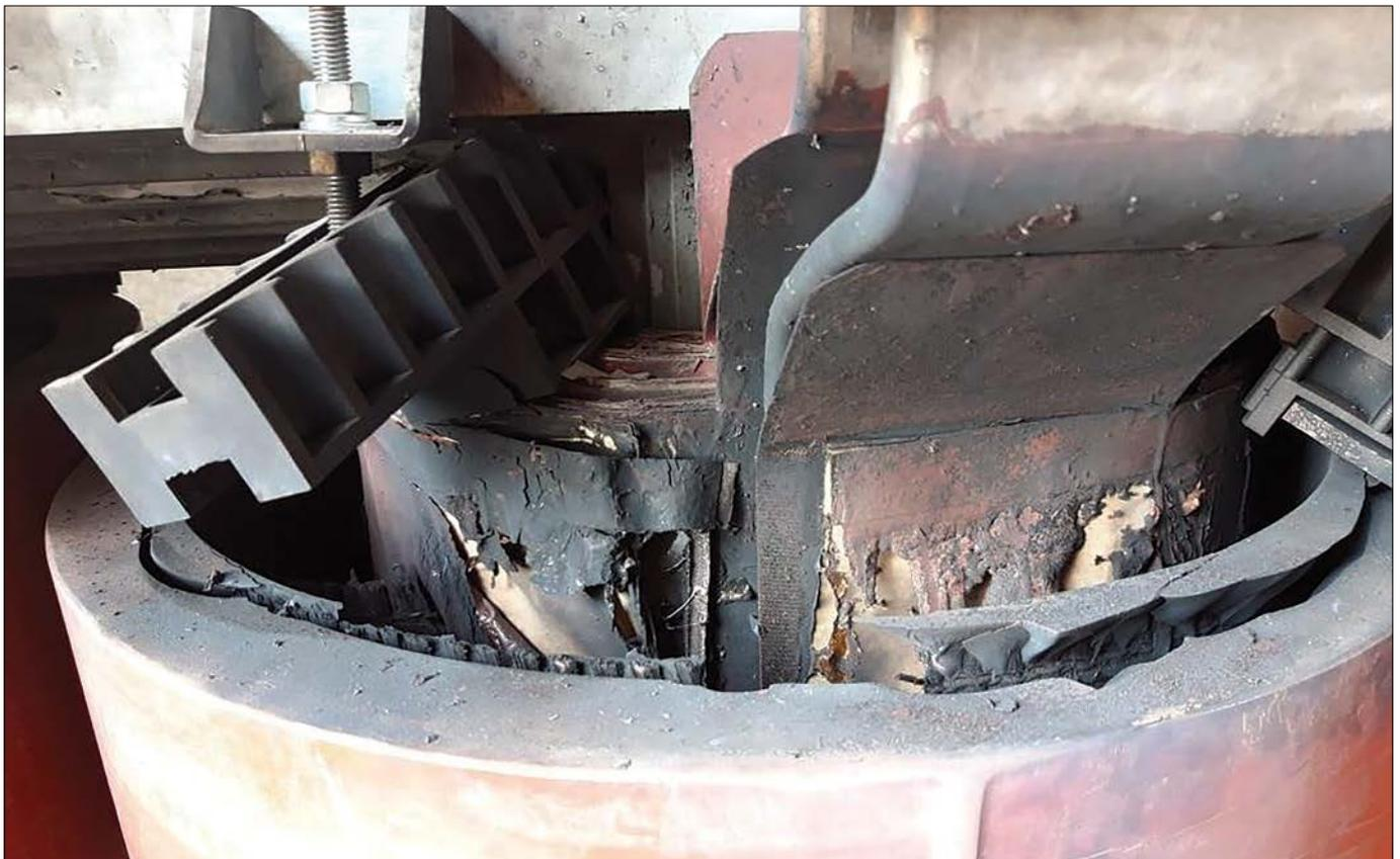
Fig. 4. The destructive effect of an electrical fault. Catastrophic discharge destroyed the central phase and charred part of the resin. The VOC sensor positioned above the phase was hit by the blow and failed.
