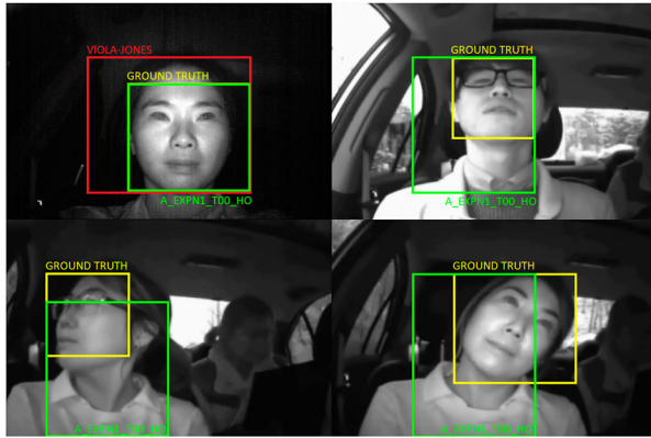
Figure 11. FADID dataset approximate face region detection examples with ground truth bounding box (yellow), proposed variant A_Expn1_T00_HO bounding box (green) and Viola-Jones bounding box (red), including the examples in which the algorithm doesn't perform well.
