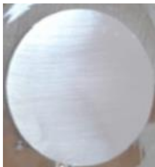
Figure 9. Surface image of three layers of waterborne acrylic coating C1 coated on a RG7 bronze where each layer was dried at 40 °C for 4 hours
