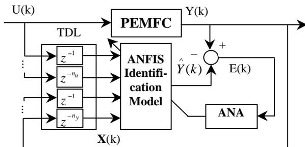
Fig. 2 Identification structure of PEMFC system with ANFIS
