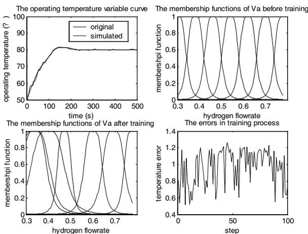
Fig. 3 Identification results of PEMFC system with ANFIS
