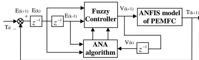
Fig. 4 Structure of adaptive fuzzy control system of PEMFC
