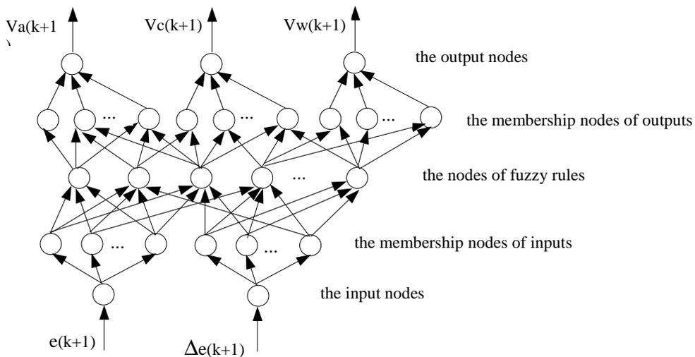
Fig. 5 Structure of the neural-networks fuzzy controller
