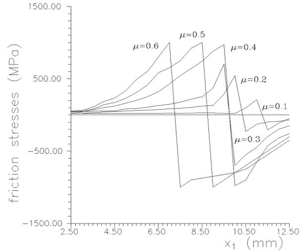
Fig. 4 Friction stresses along the contact arc
