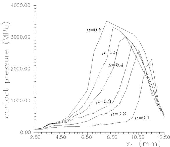
Fig. 3 Contact pressure along the contact arc
