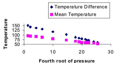
Fig. 3 Variation of temperature difference and mean temperature of air versus the fourth root of pressure
