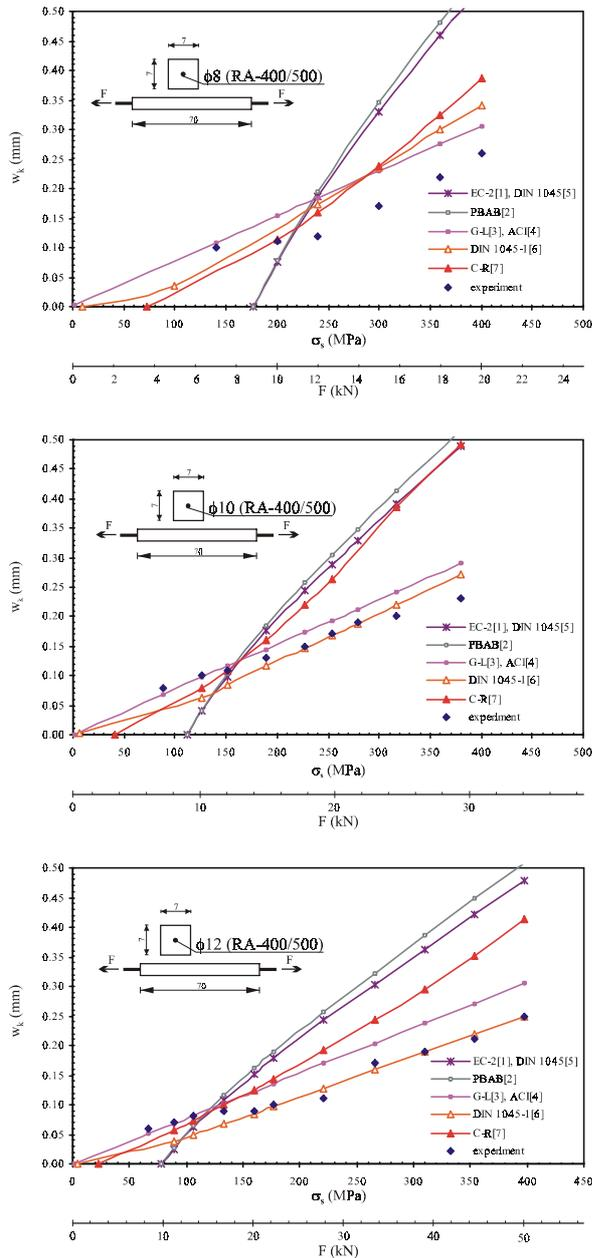
Fig. 6 Crack widths in tension elements reinforced with RA 400/500
