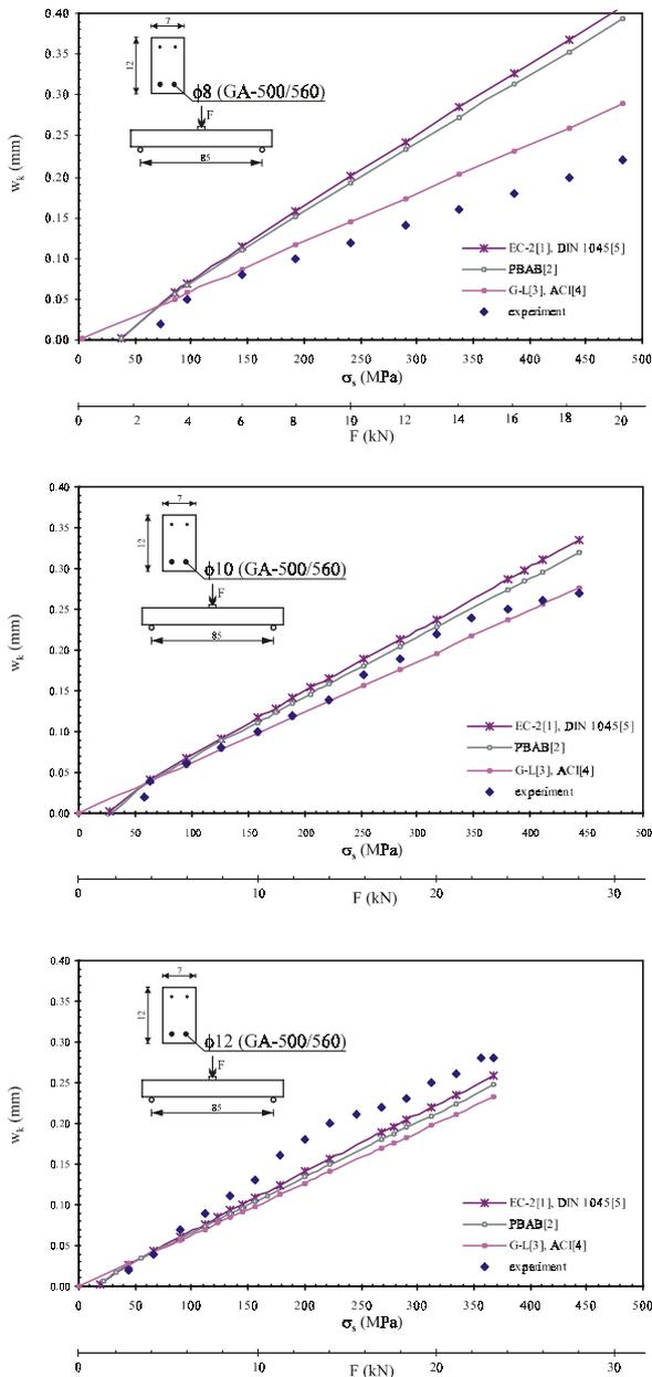
Fig. 4 Crack width for beams reinforced with GA 500/560 and exposed to bending
