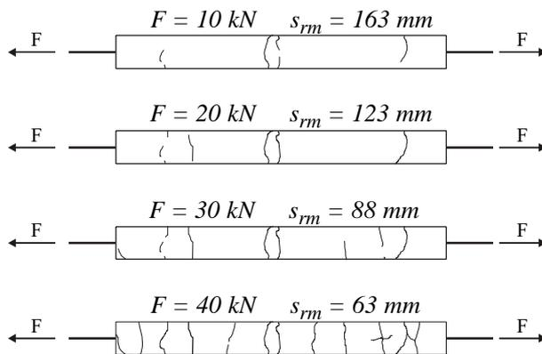
Fig. 7 Crack development in tensile element reinforced with  $\phi 12$  (RA 400/500)
