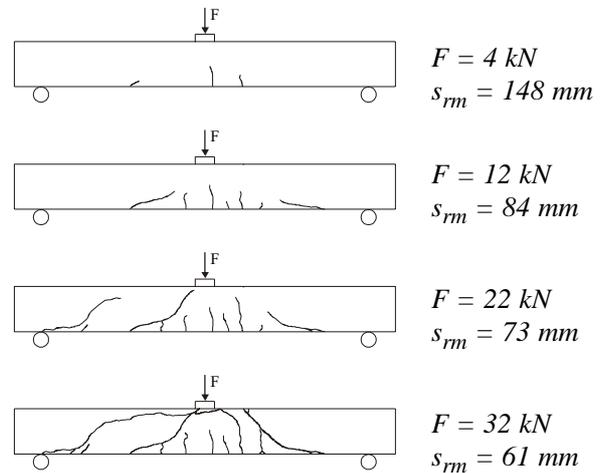
Fig. 3 Crack development in beam exposed to bending, reinforced with 2  $\phi 12$  (RA 400/500)
