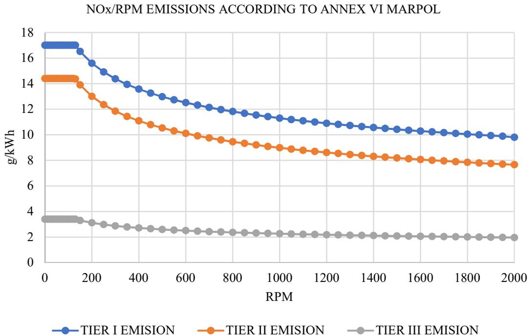
Fig. 10 NO<sub>x</sub> emission curves as a function of RPM according to Regulation 13 of MARPOL Annex VI
