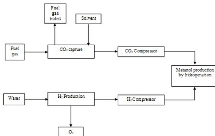
Fig. 5 Operating diagram of a hydrogenation methanol plant
