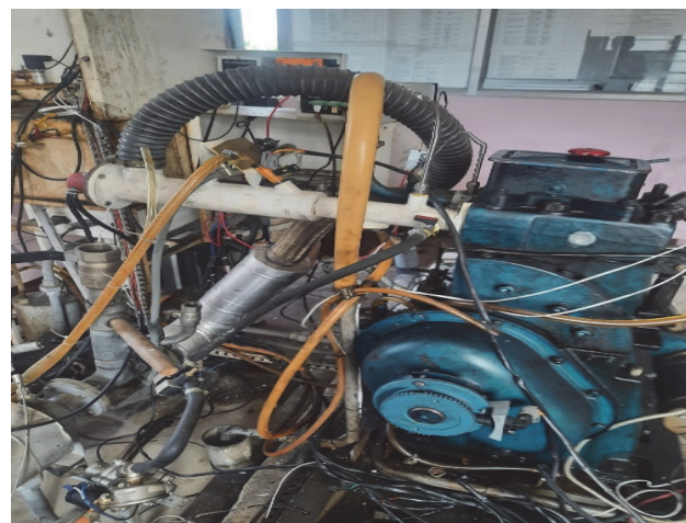
Figure 2 RCCI engine experimental setup
