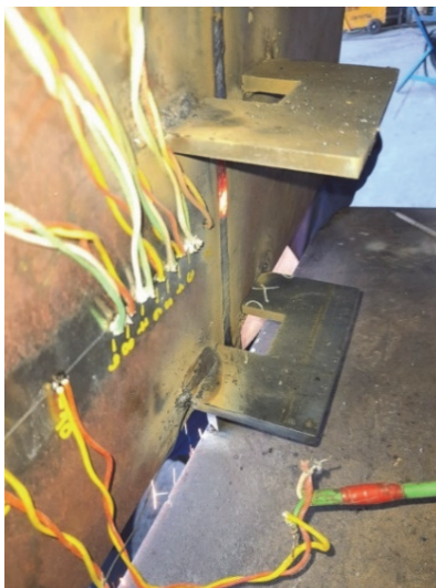
Figure 3 Temperature measurements during welding
