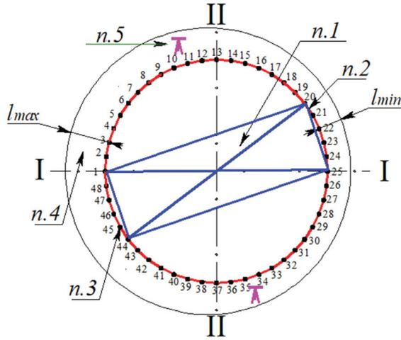
Fig. 1. Numbering of points on the under-crane track: 1 point – circular bridge crane; 2 point – circular sub-crane track; 3 point – points on the track; 4 point – service area; 5 point – “virtual stations”.
