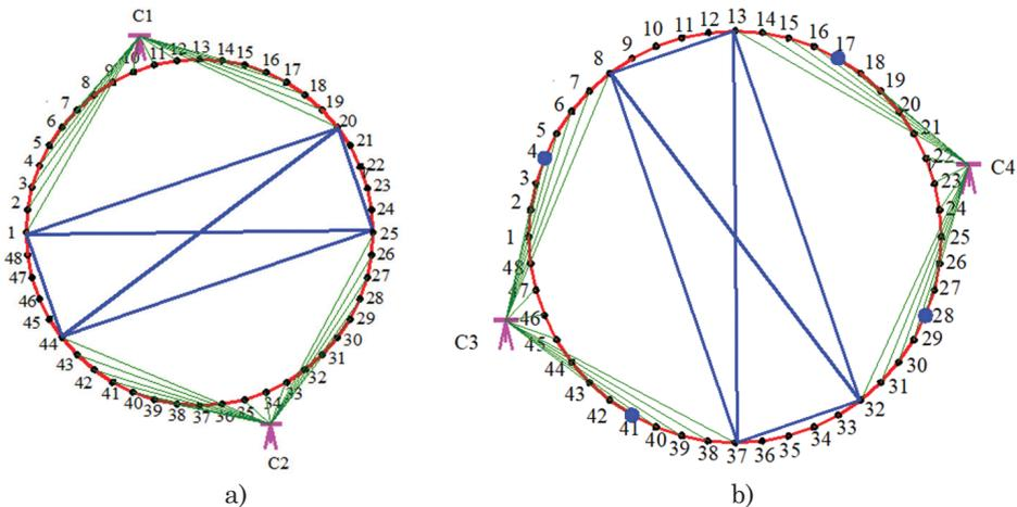
Fig. 2. Placement of a polar crane to monitor the sector a) 1÷20, 25÷43, b) 37÷8, 13÷3; C1, C2, C3, C4 – leveling stations.
