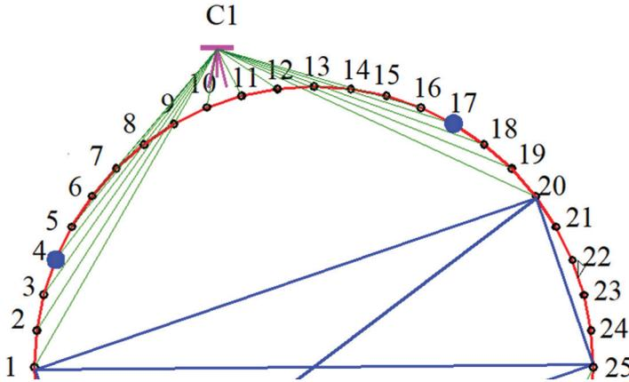
Fig. 5. Scheme of measurement by an electronic level in the sector 1=20 from station C1.
