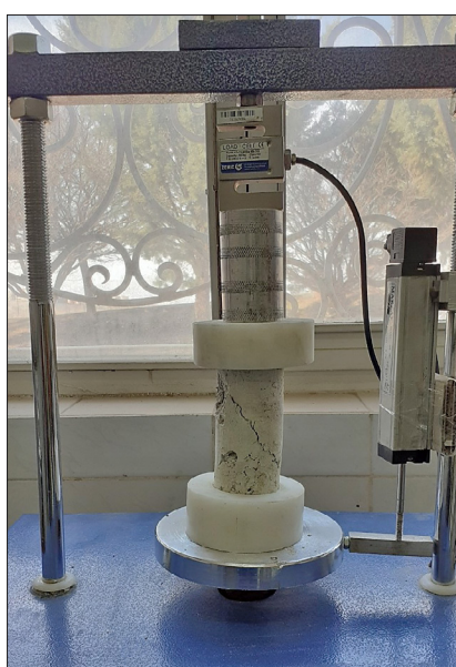
Figure 7: The fractured sample under uniaxial load
