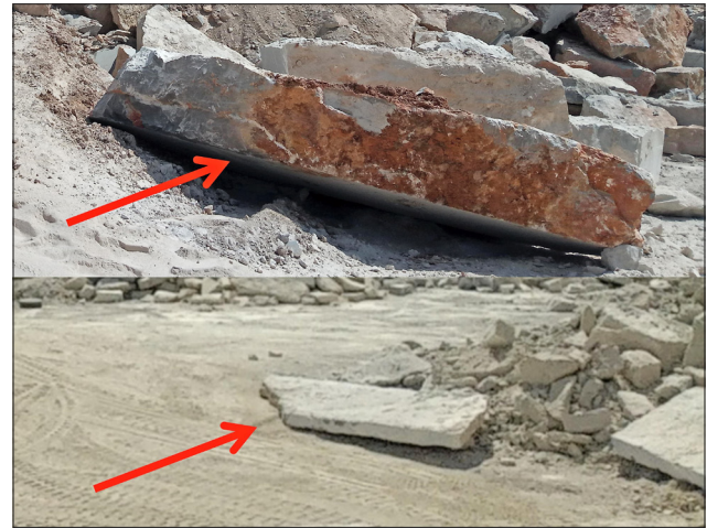
Figure 5: Examples of the formation of blocks with low height in Lashotor quarries complex
