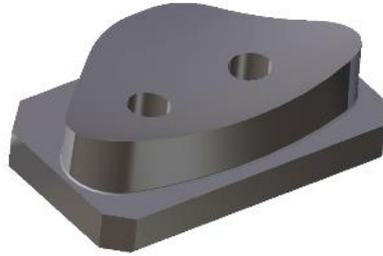
Figure 3. Punch 3D model.
