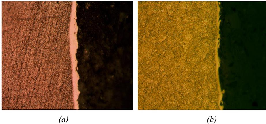
Figure 18. White layer resulting from wire erosion.
