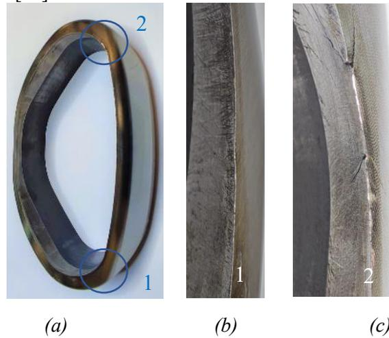
Figure 13. Deformation belongs to the matrix, whose hardness ranges from 52 to 54 HRC.
