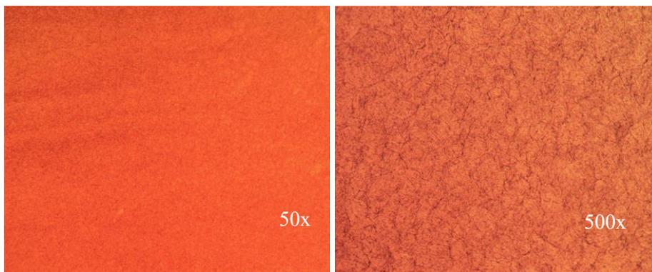
Figure 15. Matrix core microstructure (x50 and x500 magnification) for 52-54 HRC.
