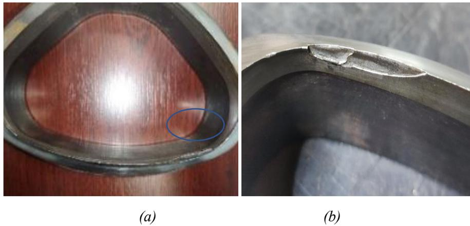
Figure 11. Deformation in matrix for 56-58 HRC.
