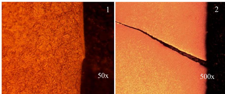
Figure 14. Matrix cutting contour microstructure (x50 and x500 magnification) for 52-54 HRC.
