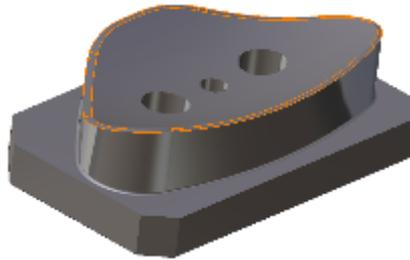
Figure 7. Flat area around the cutting edge.
