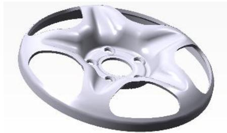
Figure 2. Disc component of wheel 3D model.
