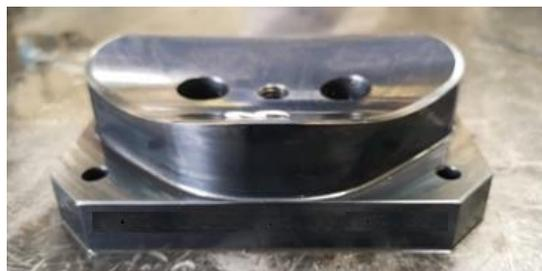
Figure 8. Punch surface coating.
