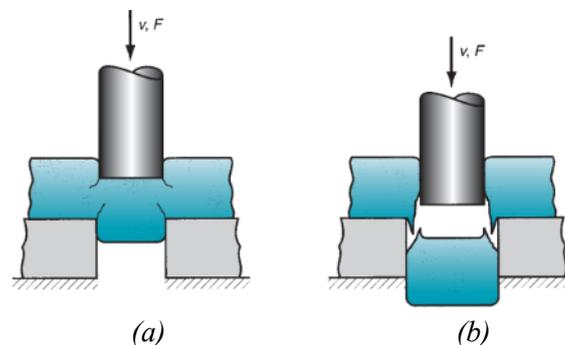
Figure 1. Effect of die clearance [4].
