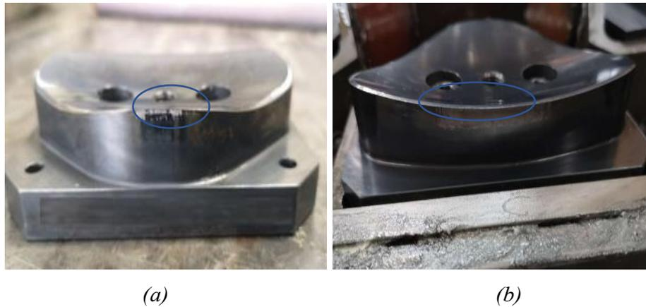
Figure 10. The deformations observed in punches from the P-2 experiment.
