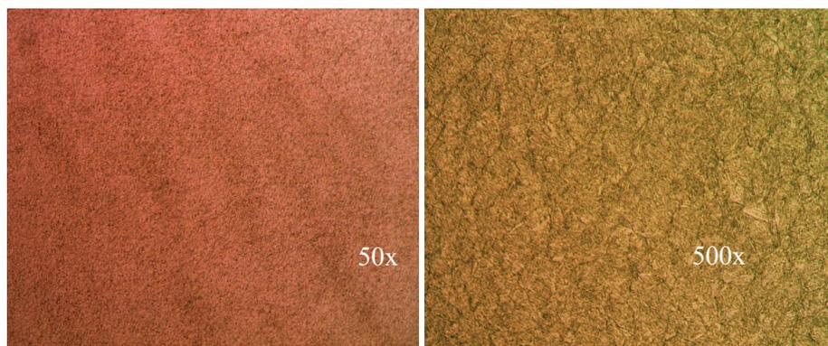
Figure 12. Matrix core microstructure (x50 and x500 magnification) for 56-58 HRC.
