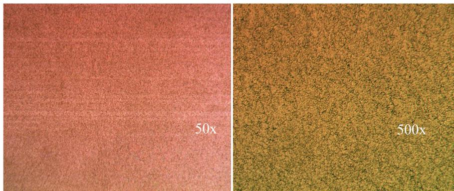
Figure 17. Matrix core microstructure (x50 and x500 magnification) for Vanadis 4 Extra.
