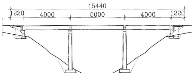
Fig. 7 Box girder bridge: longitudinal section
