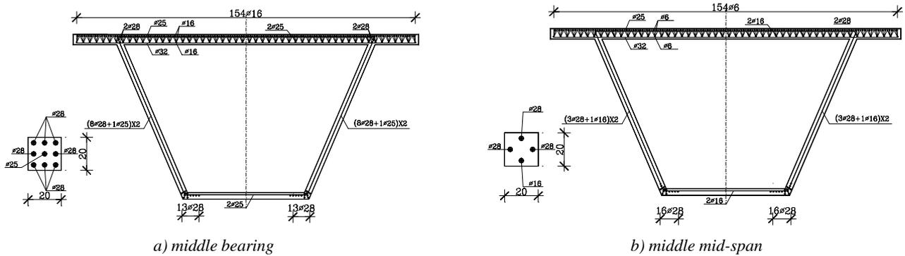
Fig. 11 Box girder reinforcement in characteristic cross-sections of the bridge
