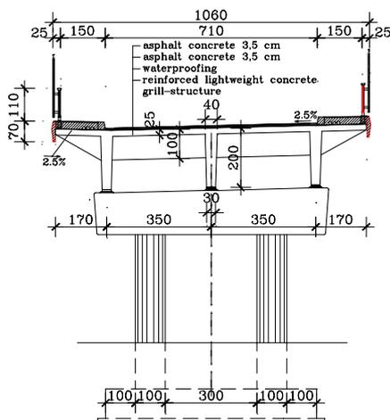
Fig. 2 Highway overpass - cross-section
