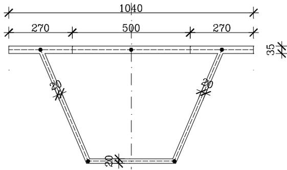
Fig. 13 Sketch of the cross-section of the box model
