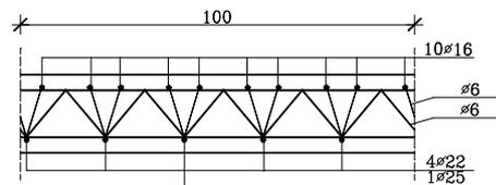
Fig. 3 Slab reinforcement of the overpass
