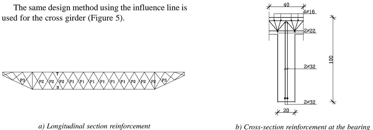
Fig. 5 Reinforcement of the cross girder
