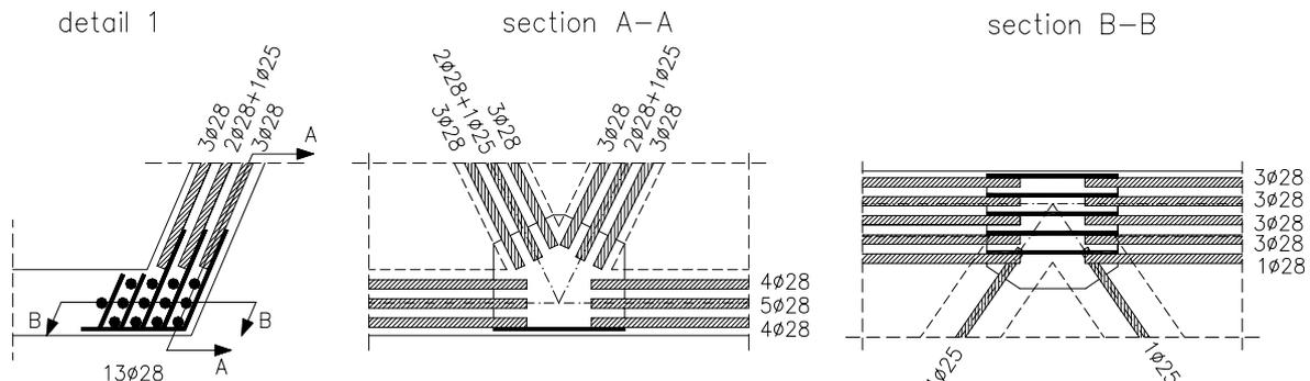
Fig. 12 Steel plates for reinforcement connection
