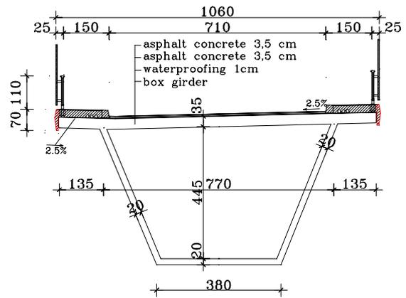
Fig. 8 Box girder bridge: cross-section of the superstructure
