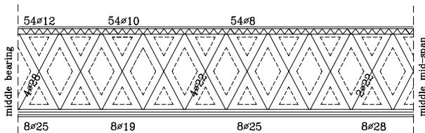
Fig. 6 Longitudinal disposition of the border main girders reinforcement in the middle field
