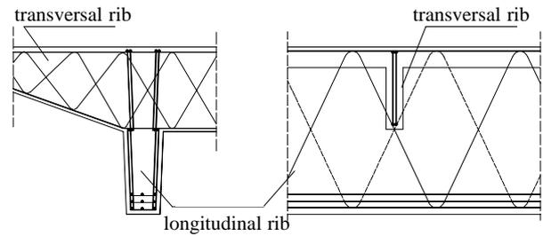
Fig. 15 Setting of longitudinal and transversal trusses
