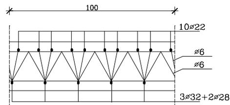
Fig. 9 Slab reinforcement of the box-girder bridge
