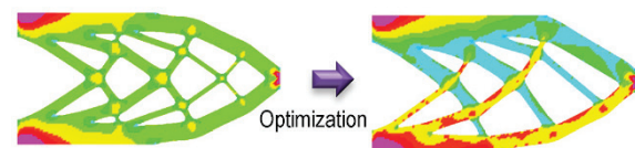
Figure 1 Higher stress in compression zones of the part
