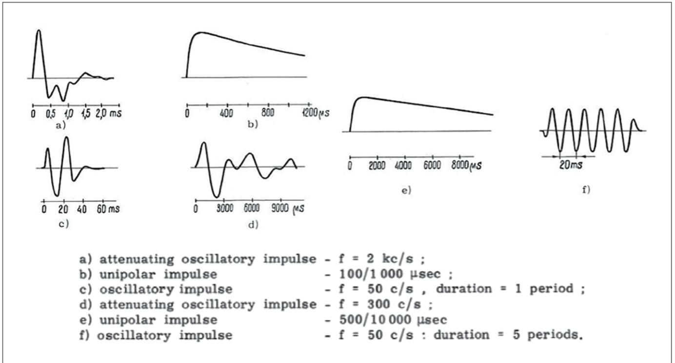
Figure 8. Oscillograms of aperiodic and oscillatory impulses simulating switching surge acc. Kaplan & Morozova = Fig. 3, CIGRE-1970 [6]
