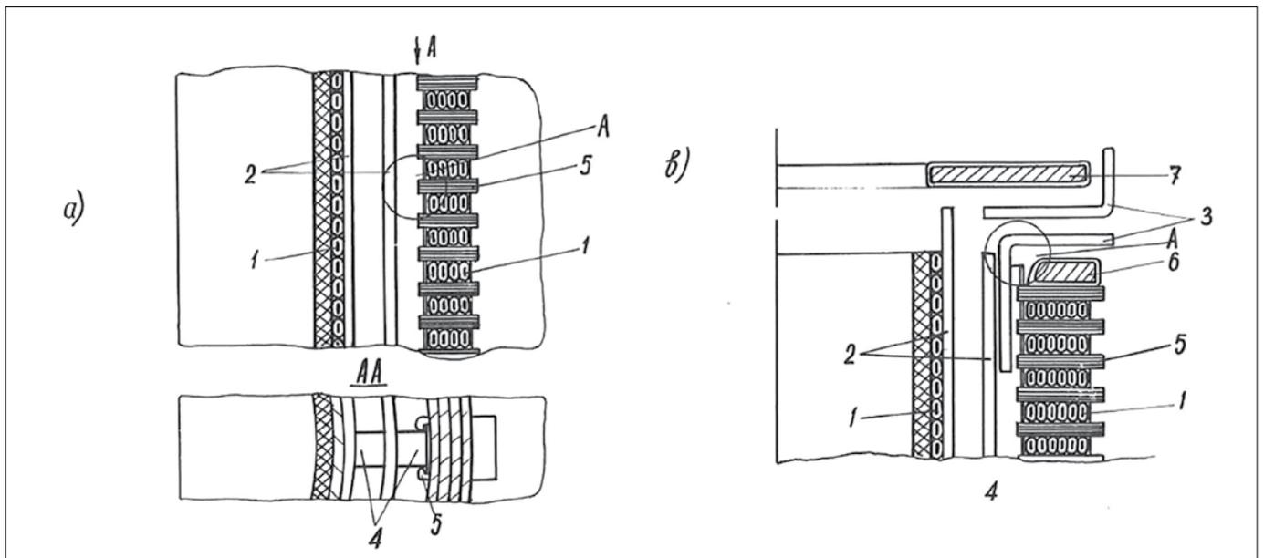
Figure 7. Model of oil-barrier insulation of the middle (a) and of the edge (b) of winding acc. Kaplan & Morozova = Fig. 1, CIGRE-1970 [6]
