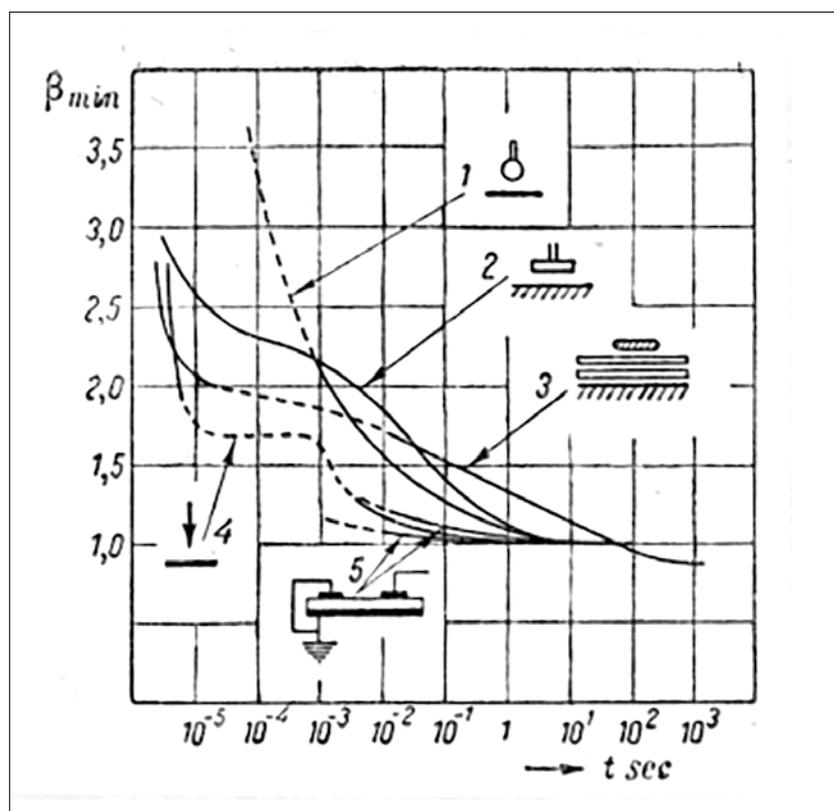
Figure 1. Volt-second characteristics of different types of oil insulation acc. to Panov = Fig. 13, Panov [1]
