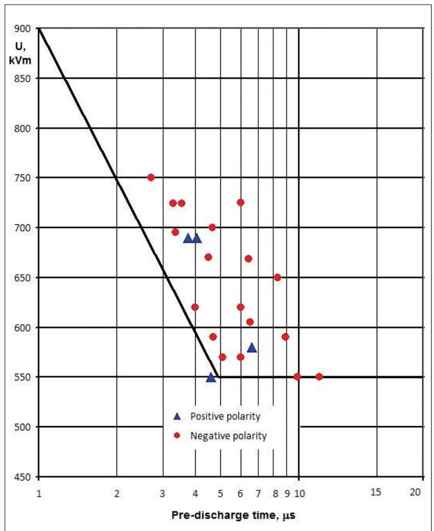
Figure 4. Volt-second characteristic of oil barrier insulation at exposure time 1 – 15  $\mu$ s, impulses 1.5/40  $\mu$ s acc. to Panov (rebuilt from Fig. 25-15 [2])
