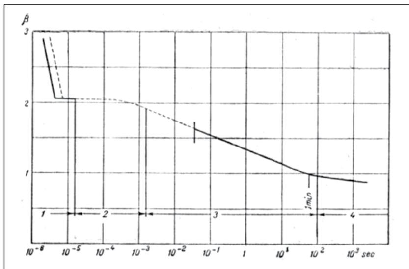
Figure 6. Volt-second dependence of the main insulation between the HV and LV windings acc. to Panov = Fig. 12, Panov [1]
