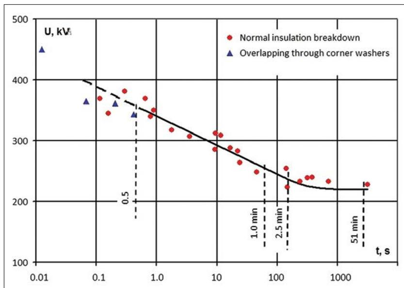
Figure 5. Volt-second characteristic of oil barrier insulation at the exposure time 0.1 sec - 51 min., 50 Hz acc. to Panov (rebuilt from Fig. 25-14 [2])
