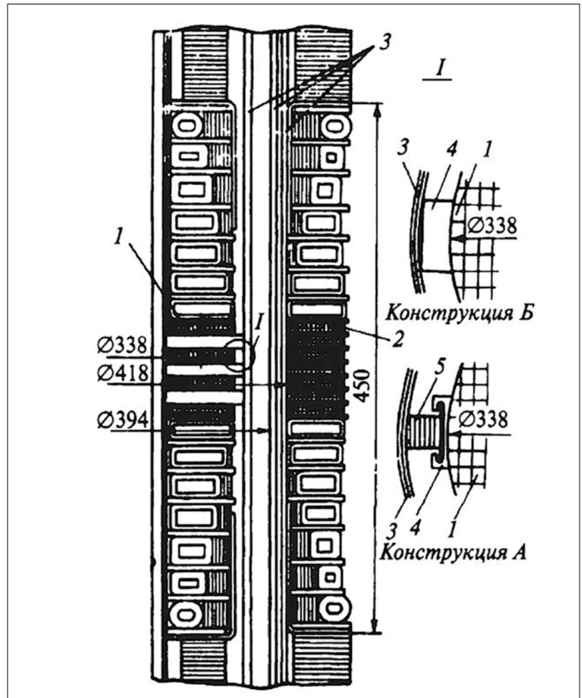
Figure 11. Model of the main insulation with an input in the middle of the winding (MKI) acc. Morozova-1977
