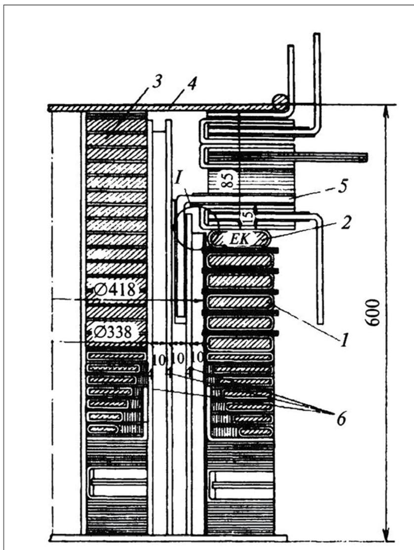
Figure 12. Model of the main insulation with an entry at the end of the winding (MKI) acc. Morozova-1977
