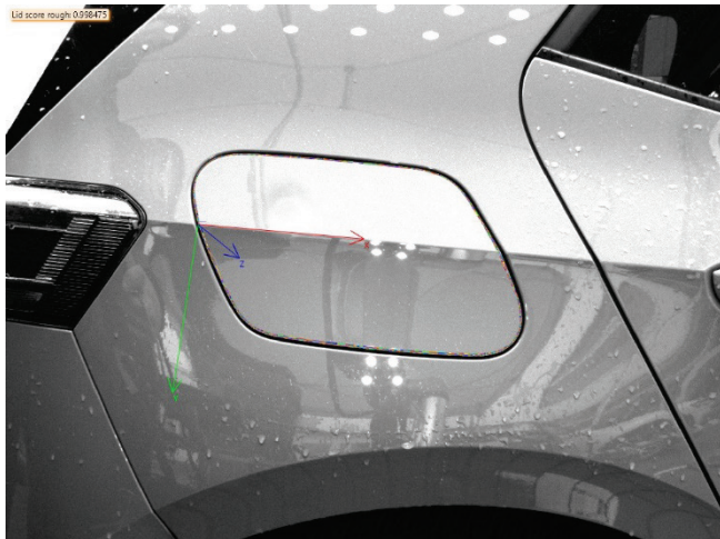
Figure 5 Position determination of a VW ID3 charging lid
