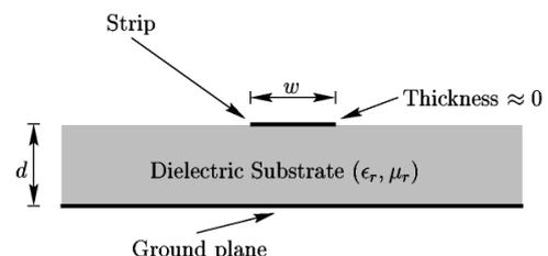
Fig. 9 Infinite microstrip line for two-dimensional version of SDM
