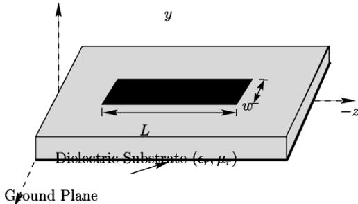
Fig. 7 Microstrip resonator
