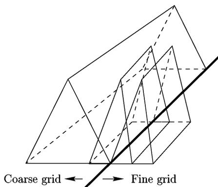
Fig. 4 Connection of coarse and fine grids
