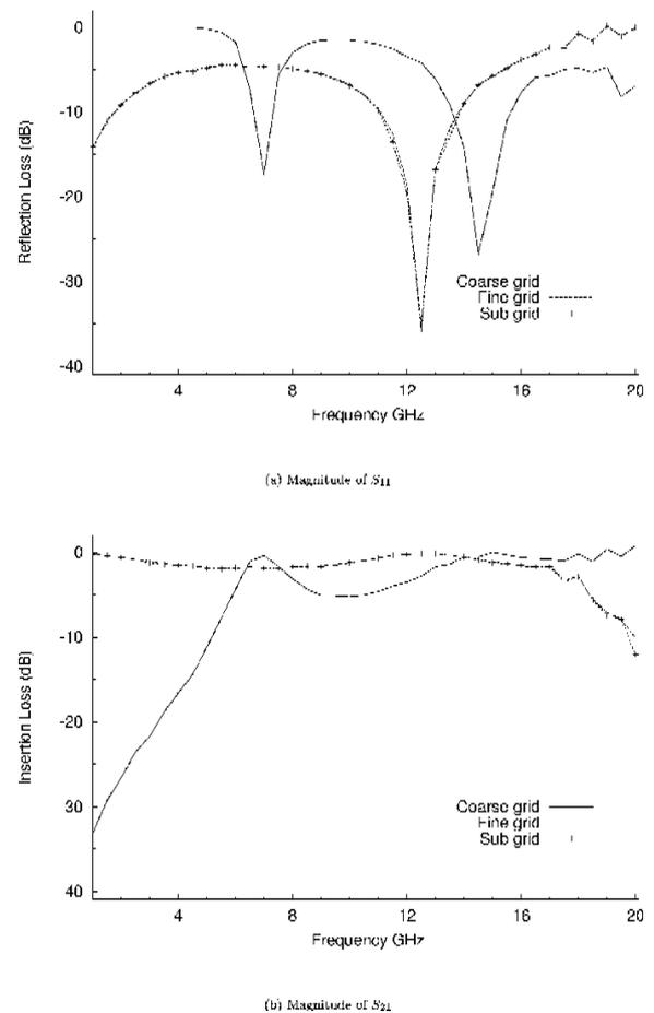
Fig. 20 Plot of S-parameters' magnitude for the step discontinuity
