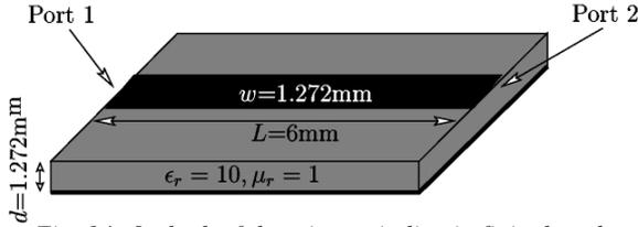
Fig. 14 Outlook of the microstrip line in finite length
