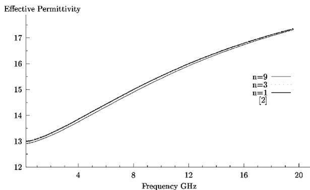
Fig. 10 Dispersion characteristics for the open infinite microstrip line
