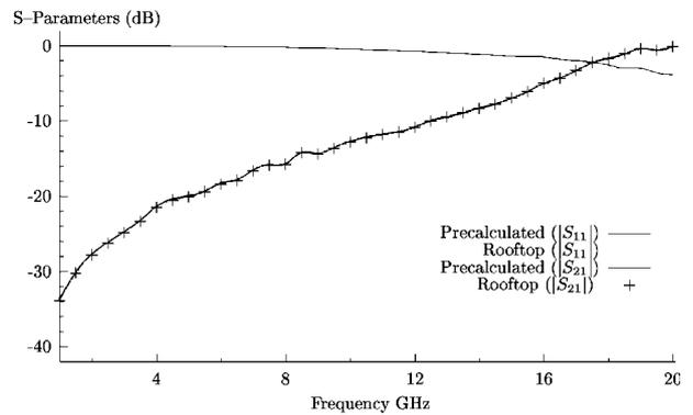
Fig. 13 Plot of S-parameters's magnitude for the microstrip gap discontinuity comparing basis function sets
