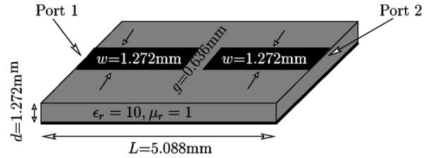
Fig. 12 Microstrip gap layout
