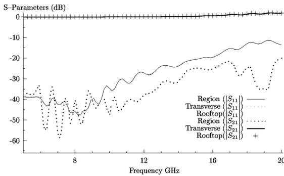
Fig. 15 S-parameters' magnitude for the microstrip line
