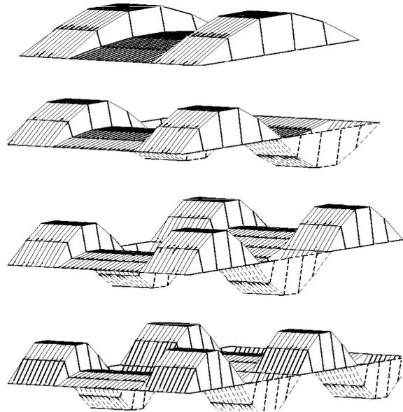
Fig. 17 Current distributions for the first four resonant modes of a strip resonator
