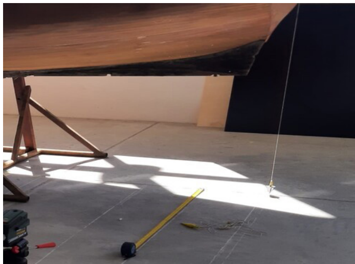
Figure 4: Using measurement tools for point on the sections
