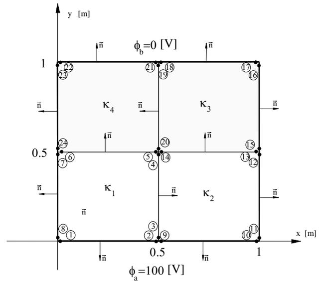
Fig. 5 Heterogeneous domain divided into four homogeneous sub-domains
