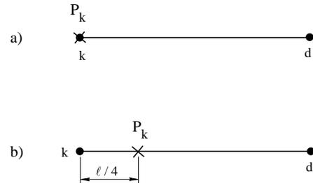
Fig. 3 Location of the collocation point  $P_k$  joined to the  $k$ -th node
