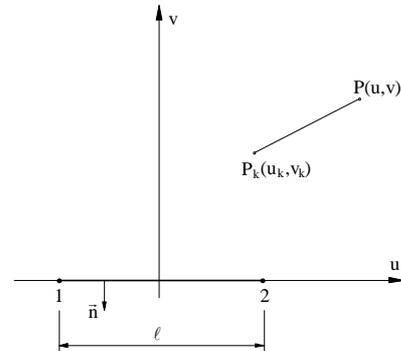
Fig. 2 Linear boundary element in the local co-ordinate system
