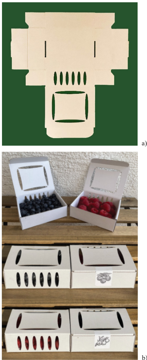
Figure 3. a) Photo of the overcut of the packaging, b) Photo of the finished prototype
